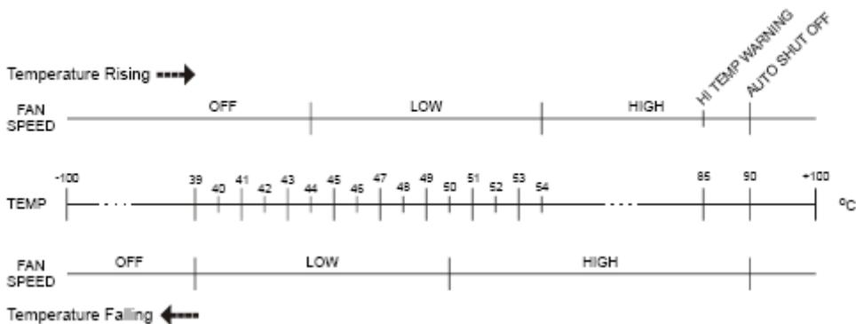
**Figure A-1.** Fan Speed vs. Temperature
