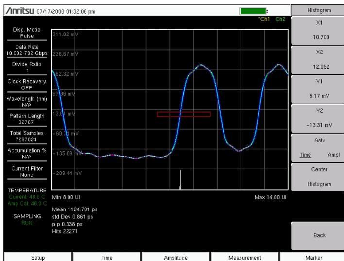
Figure 4-3. Pulse pattern display with a histogram measurement.
