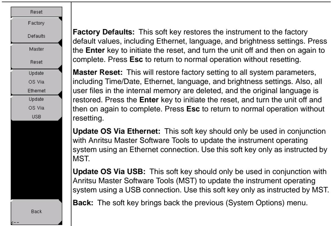
**Figure 4-39.** Reset Submenu
