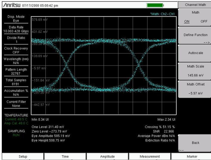
Figure 4-6. Channel Math Result for the Ch2-Ch1 Function
