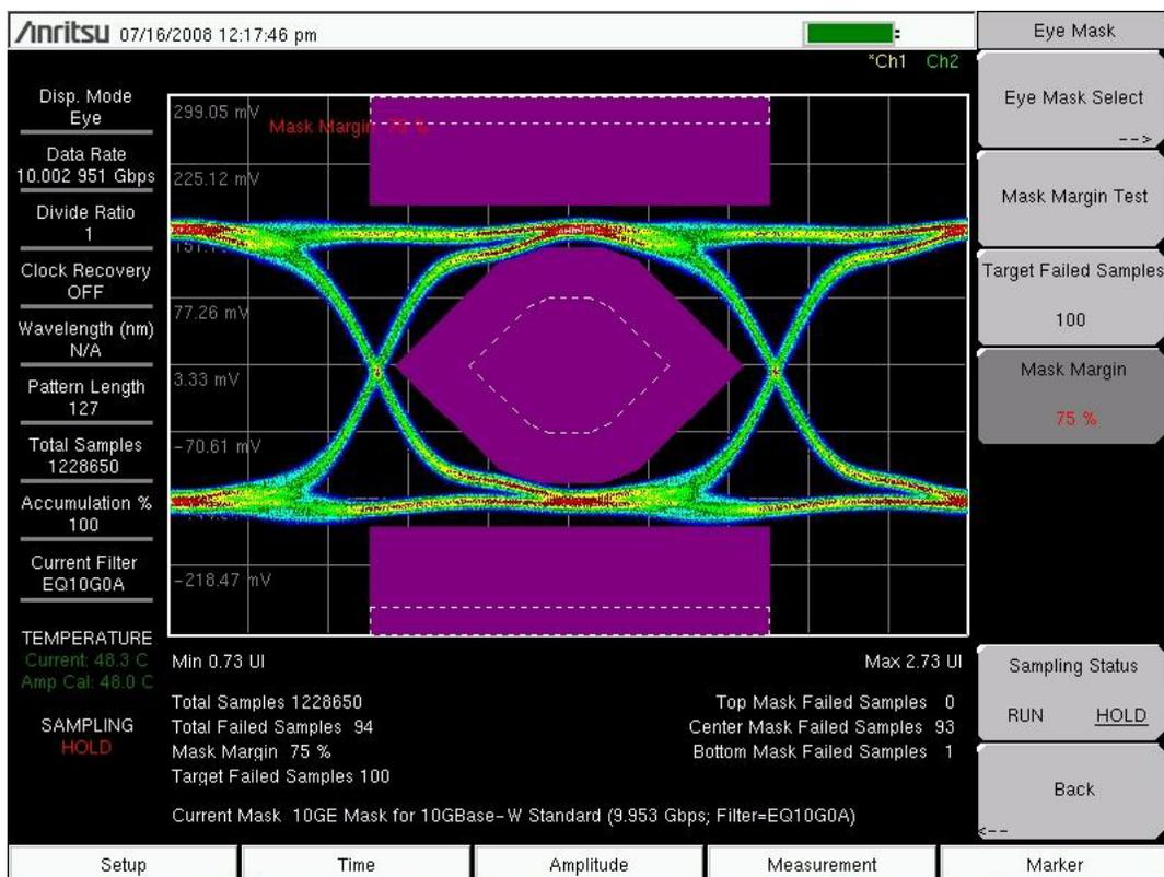
**Figure 5-8.** Mask Margin Measurement on Eye Pattern Display
