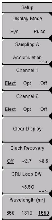
**Clock Recovery:** The Clock Recovery soft key allows the selection of the settings of the clock recovery function. The clock recovery can be set to the band <2.7 (0.1 – 2.7 GHz), or to the band >8.5 (8.5 – 12.5 GHz). The clock recovery function can also be turned Off. Choose the appropriate setting based upon the data rate of the input data pattern. The <2.7 and >8.5 choices are available only with Option 002.
