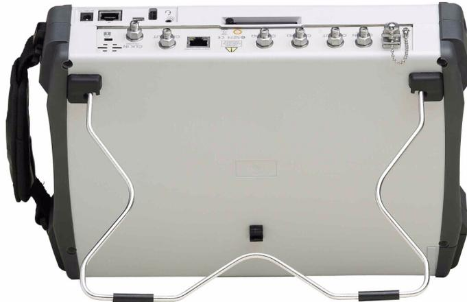
**Figure 1-4.** Tilt Bail Extended on the Bit Master
