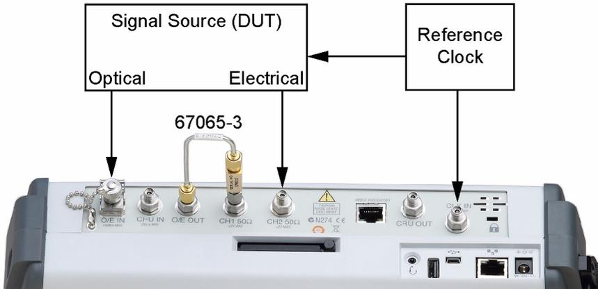
**Figure 3-3.** Making Connections Using Optical Data and Electrical Clock.
