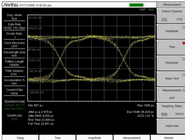
Figure 4-1. Eye pattern measurement display with no accumulation.
