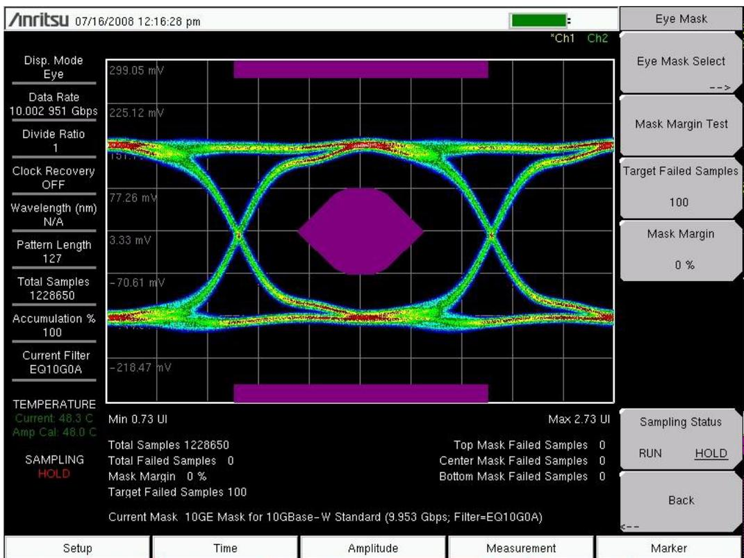
Figure 5-7. Mask Measurement on Eye Pattern Display.
