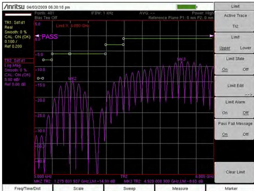
**Figure 14-2.** Differential  $S_{11}$  Log Magnitude Display of  $S_{d1d1}$
