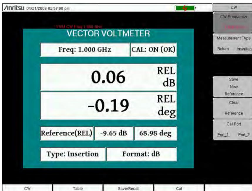
**Figure 11-5.** Continuous Wave Menu with Relative Measurements
