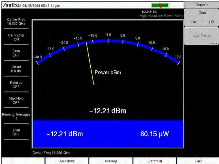
**Figure 12-2.** Power Meter Display and Zero/Cal Menu
