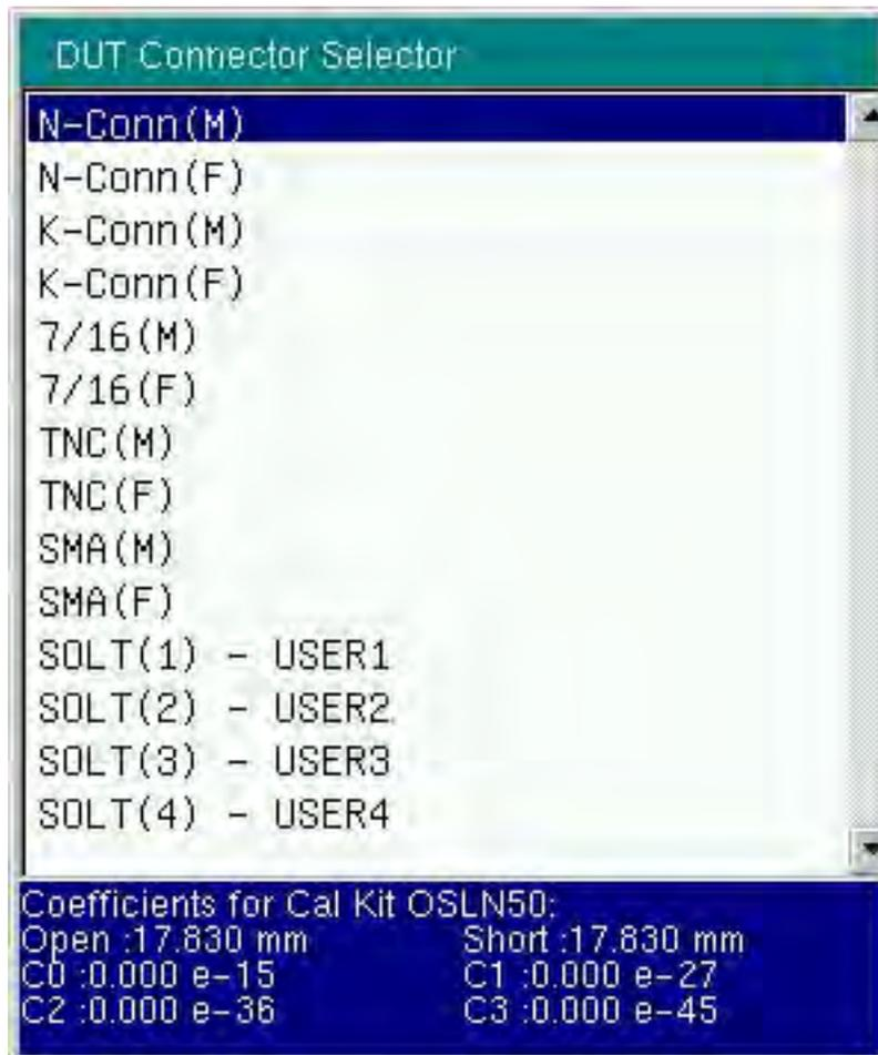
**Figure 6-16.** DUT Connector Selector List Box for Cable
