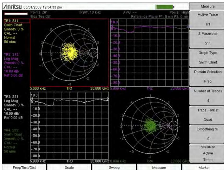
Figure 2-4. 4 Traces in 4 Window Images (Quad Trace Format)
