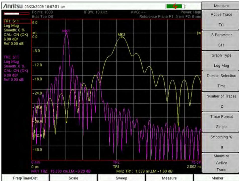
Figure 5-12.  $S_{11}$  on 15 cm Shorted Waveguide Section
