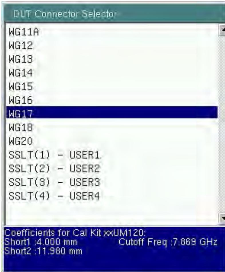
**Figure 6-19.** DUT Connector Selector List Box for Waveguide
