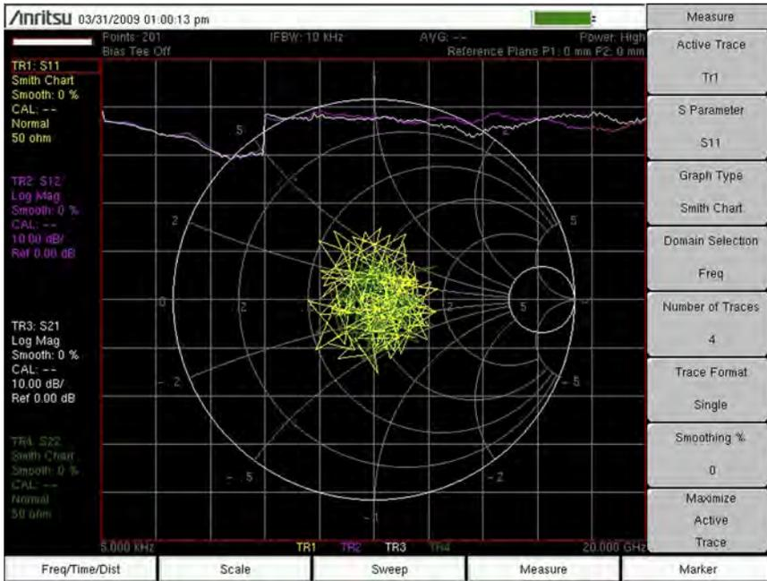
Figure 2-5. 4 Traces in 1 Window Image (Single Trace Format)
