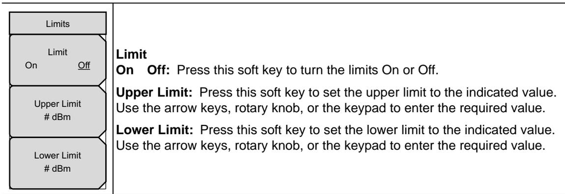
**Figure 12-11.** Amplitude and Units Soft Key Menus
