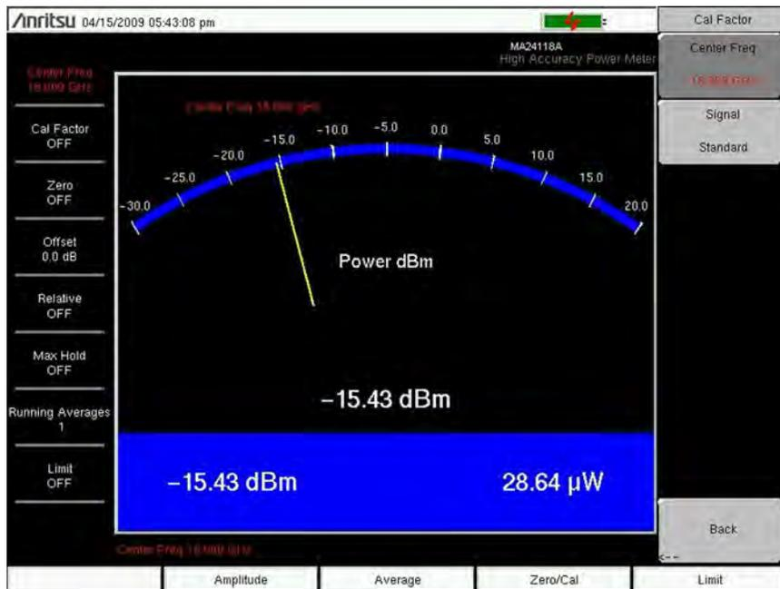
**Figure 12-3.** Power Meter Display and Cal Factor Menu
