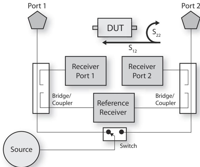
**Figure 4-2.** MS202xB VNA Master Block Diagram During Reverse Sweep
