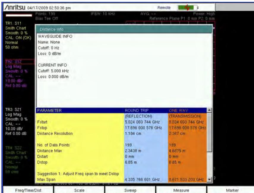
Figure 6-10. Distance Information List Box for Waveguide
