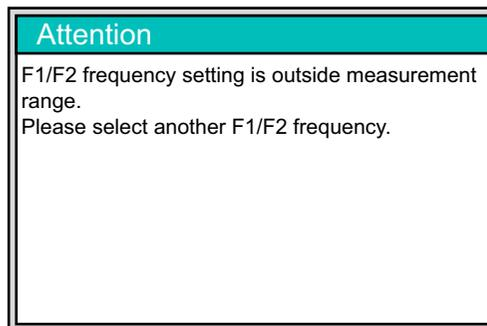
**Figure 2-3.** Carrier F1 or Carrier F2 Outside Frequency Range Error Message
