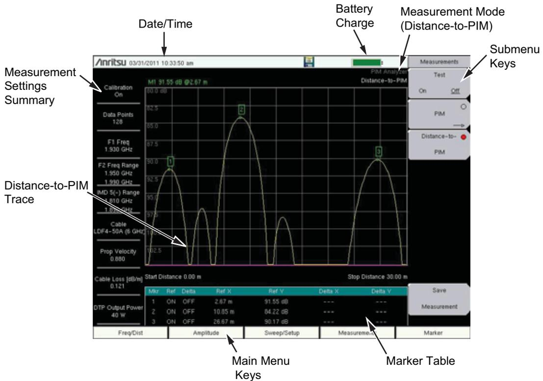
Figure 1-4. Distance-to-PIM Analyzer Display
