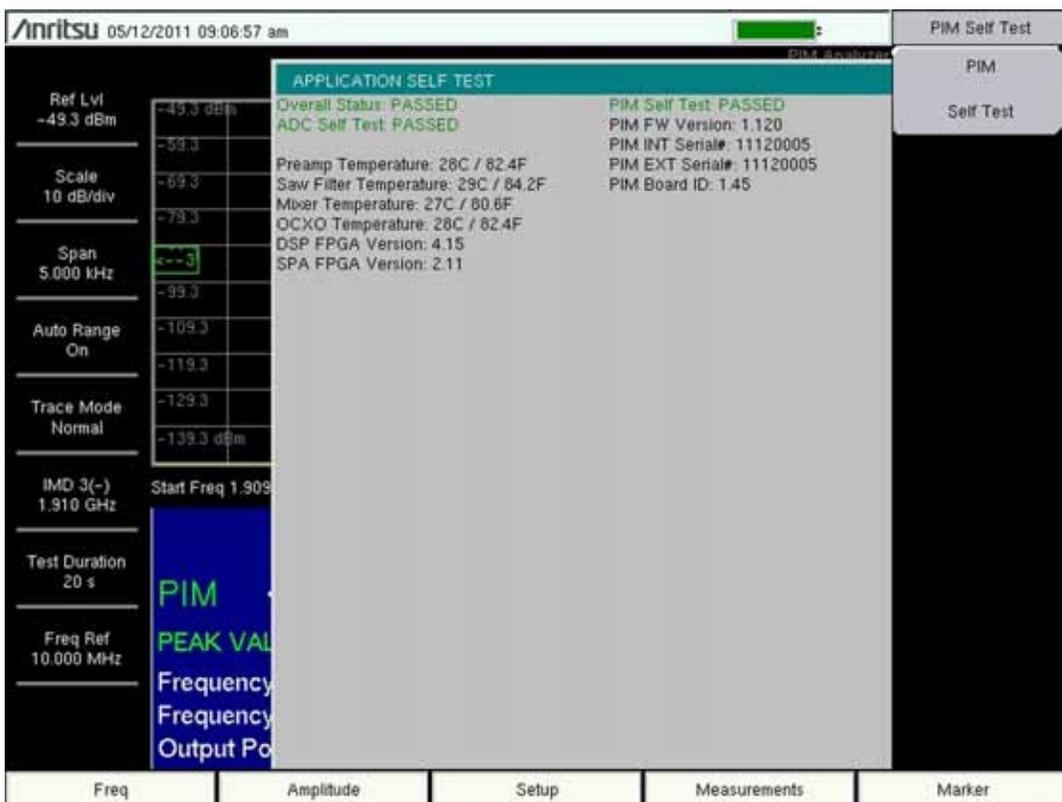
**Figure 1-5.** PIM Self Test Displays Firmware Version
