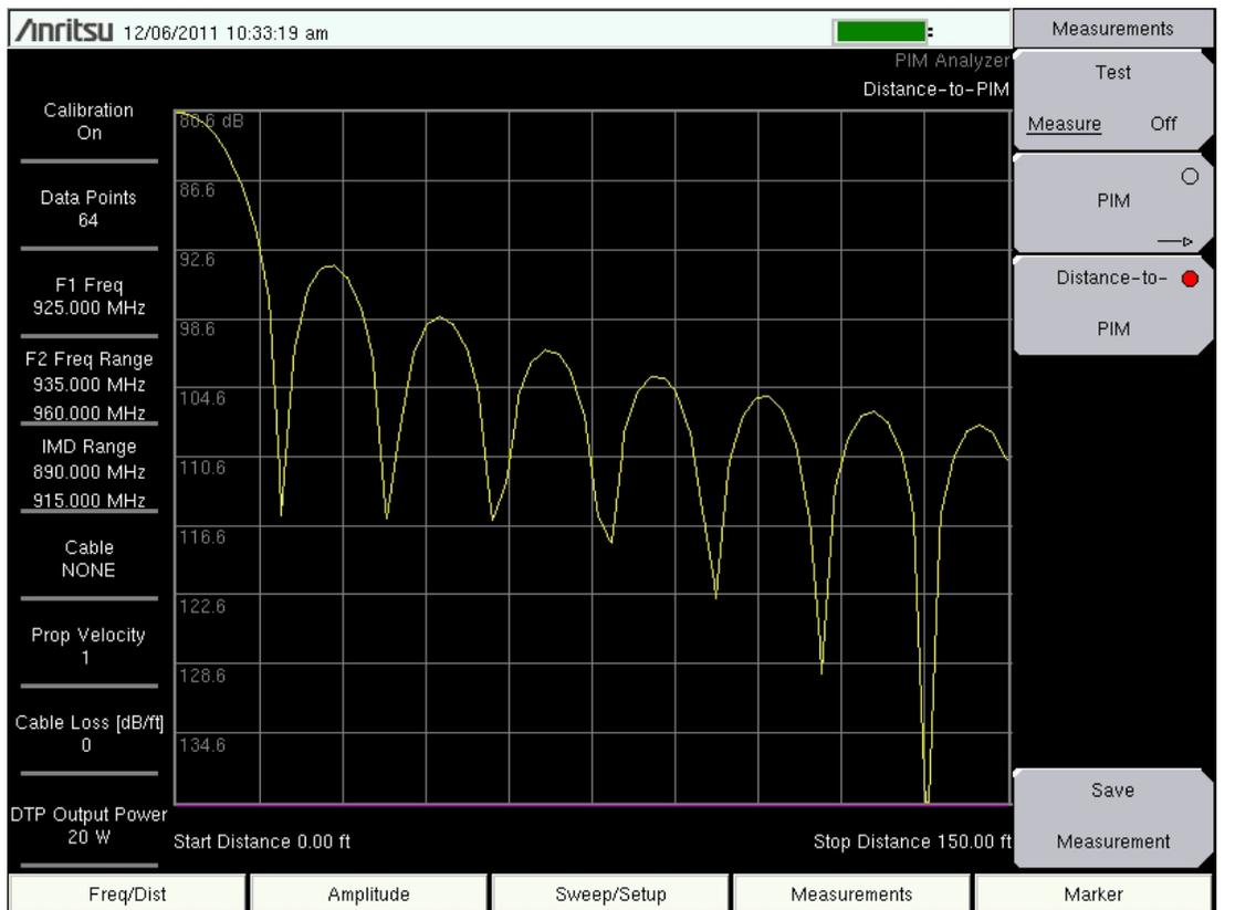
**Figure 3-2.** Typical DTP Measurement After a Calibration
