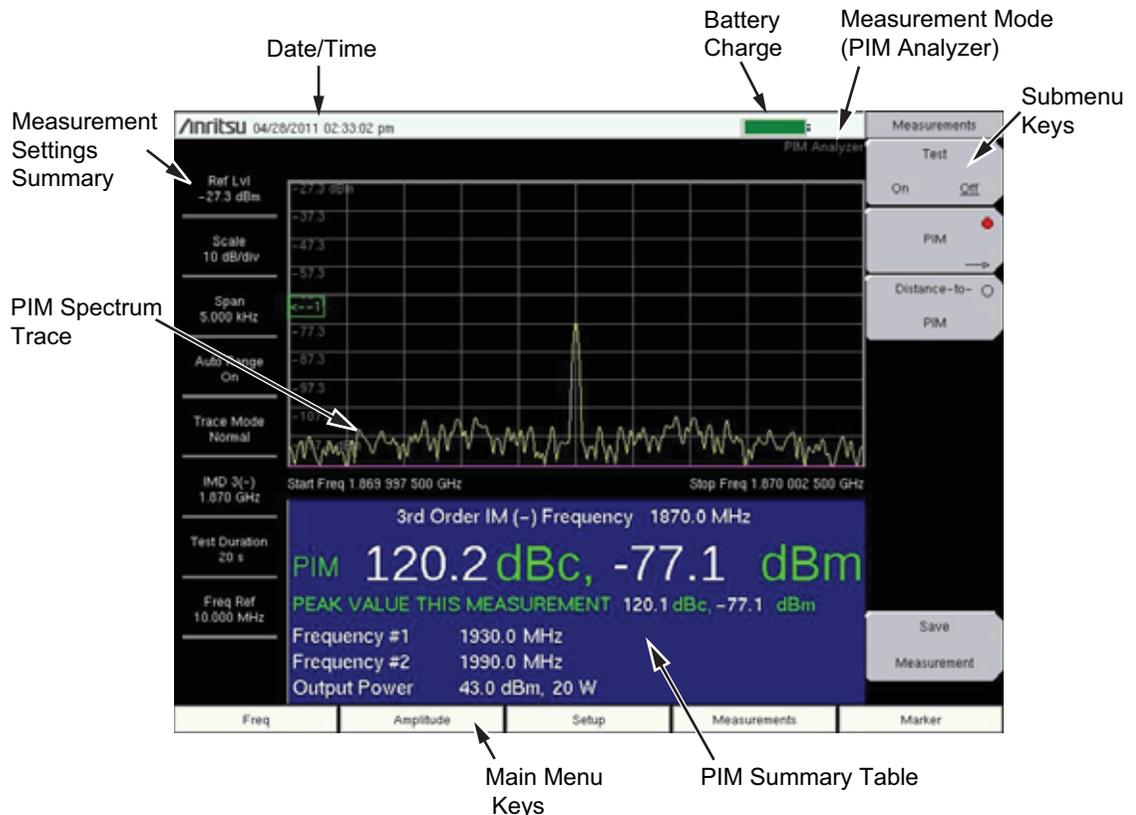
Figure 1-3. PIM Analyzer Display
