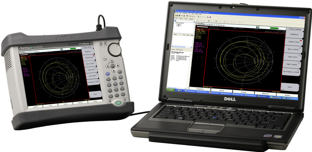
Figure 2-9. MS2035B Connected to PC via USB Mini-B
