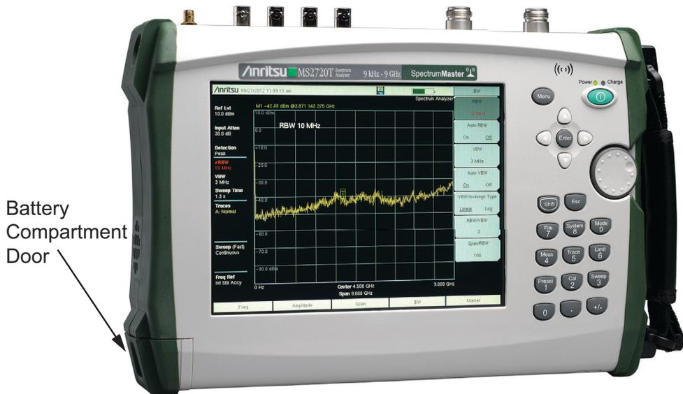
**Figure 1-1.** Battery Compartment Door
