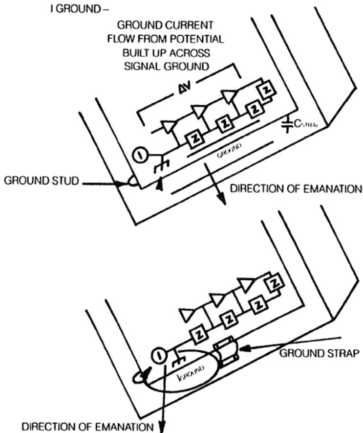
**Figure 2-9.** Changing the Geometry of Ground Straps
