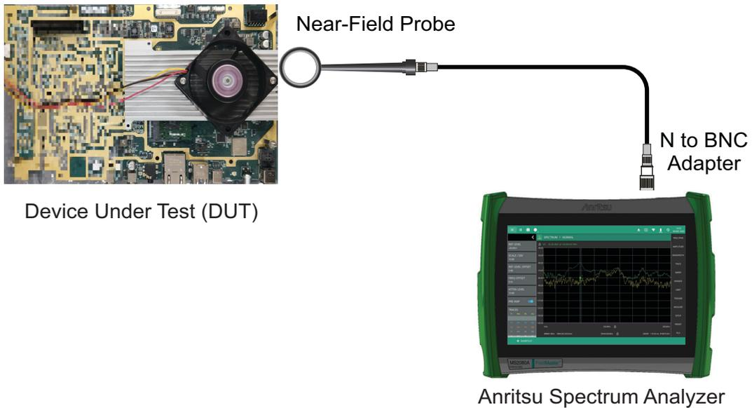
**Figure 1-2.** Typical Setup
