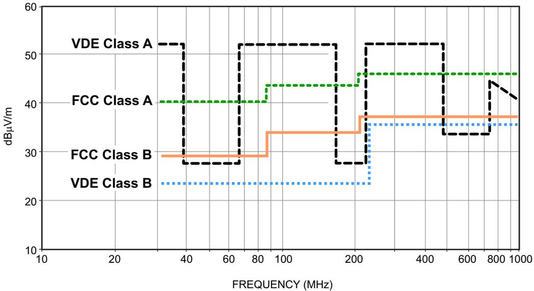
**Figure 2-1.** Conducted Noise Emissions Standards
