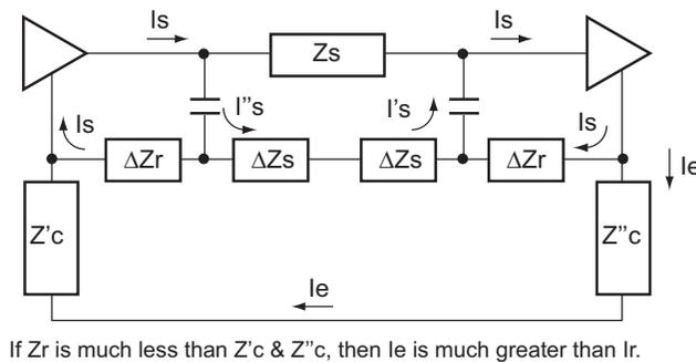
**Figure 2-4.** Comparison Between Common and Differential Current Flow
