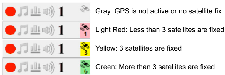
Figure 1-10. GPS Satellite Fix Indicator
