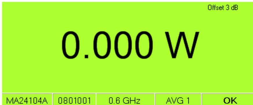
**Figure 3-5.** Display Window (Normal mode with Offset Table On)
