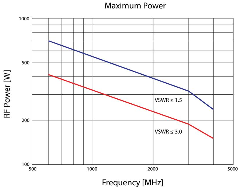
**Figure 3-21.** Maximum Power Handling Capacity (with Load VSWR less than 1.5:1 and 3.0:1)
