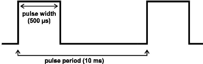
In normal measurement mode the ML2430A power meter measures and displays average power. When the signal to be measured is a repetitive pulse, an average power reading will display average power over time and not the pulse power. By entering the duty cycle of the pulse, the meter can mathematically correct to display the pulse power. This technique assumes rectangular pulses with flat pulse tops.
