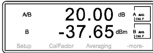
Note the small signal gain of the amplifier. Now increase the signal source power slowly. When the amplifier begins to compress the displayed gain will start to decrease. Increase the source power until the gain has dropped by 1 dB, in this example to 19 dB.
