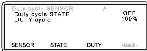
Press **[STATE]** and toggle the setting by pressing the soft key until the display reads ON. Press **[DUTY]** and using the keypad, input a duty cycle of 5%. Press **[Enter]**. To return to the Measurement screen press any hard key.
