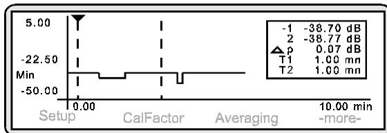
**Max** This looks at all the measurements within the block of time and returns the maximum power. The Measurement screen is similar to that achieved with Min.
