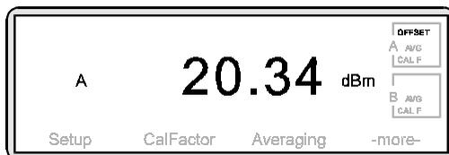
Note that box A in the top right hand corner of the screen now indicates that an OFFSET has been applied to the Sensor.
