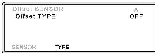
To apply an offset, press **[TYPE]**. Toggle this setting until the offset you require is displayed (see below).
