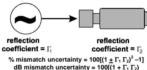
***Mismatch is easily calculated in either dB or percentage terms from the source's and sensor's respective reflection coefficients***
