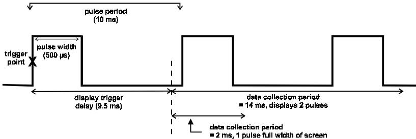
Display trigger delay is a time delay from the trigger point to the time when the power meter starts to collect data. It can be used to view the complete rising edge of a pulse which would otherwise be on the extreme left of the instrument display.
