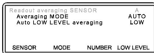
This screen reflects the default factory setting. To change the averaging mode, press **[MODE]**. Toggle this setting until the mode you require is displayed.
