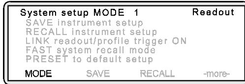
Press **[MODE]** and toggle this setting until “Power v Time” is displayed. Press any hard key to display the Measurement screen.
