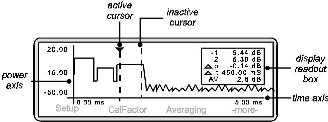
The frame is displayed on the screen and the display readout box on the right-hand side shows:
