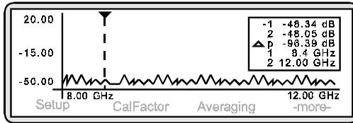
Note that the frequency axis reflects the Start and Stop settings. Each time you measure at different frequencies, it is necessary to re-input the **[START]** and **[STOP]** values.
