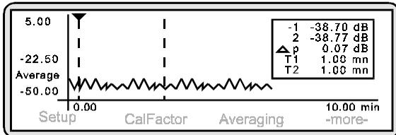
*Min* This looks at all the measurements within the block of time and returns the minimum power.
