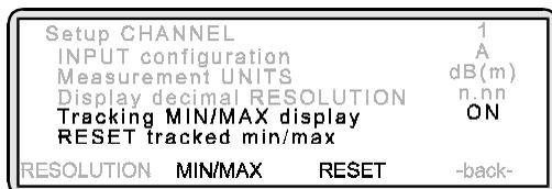
You will notice the new line “RESET tracked min/max.” The Min/Max feature can be reset to record a new time frame at any point — just select **[RESET]** from the Channel Set Up options. To return to the Measurement screen, press any hard key.
