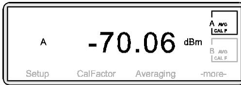
*Typical display for measurement of low power levels*
