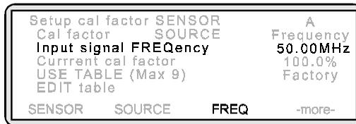
Some text on the screen appears in upper case. This indicates which soft key to select to change the item's setting. For example, to change the Input signal FREQUENCY, press the FREQ soft key.
