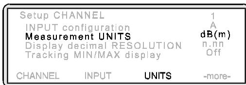
To change the resolution, press **[-more-]** to display further soft keys and then press **[RESOLUTION]**. Toggle this setting until the resolution you require is displayed.
