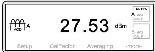
Note that box A in the top right hand corner of the screen now indicates that a Duty Cycle percentage has been applied to the Sensor.
