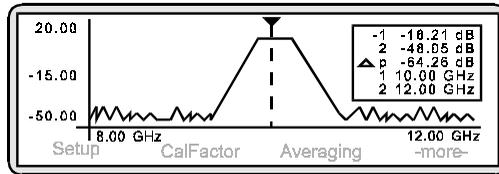
The response of the device under test is displayed on the screen and the display readout box on the right-hand side shows:
