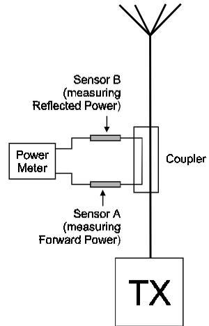
An offset has been applied to compensate for the coupling factor of the through line coupler.
