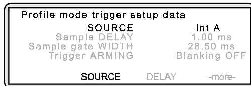
Press **[SOURCE]** and toggle this setting until the trigger source you require is displayed:
