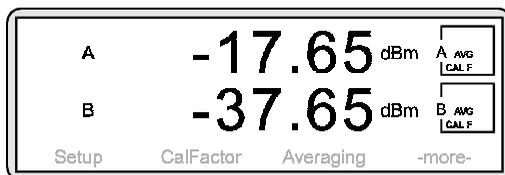
A is displaying the output power of the amplifier. B is displaying the input power to the amplifier. (Note a signal splitter has a nominal path loss of 6 dB.)
