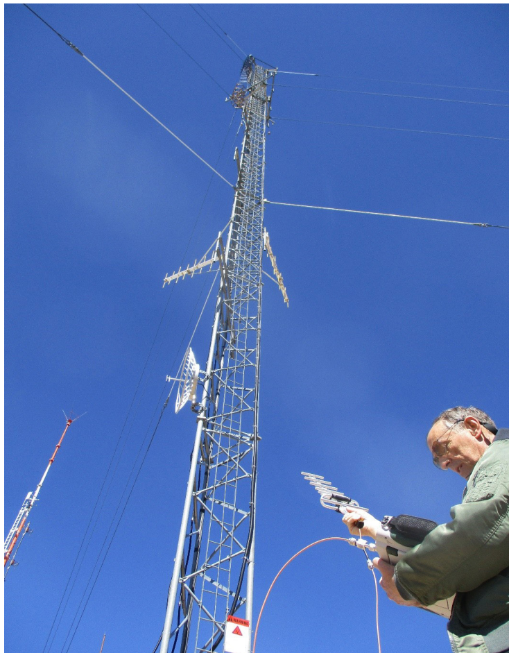
Figure 9. Using a Yagi antenna to search for the source of the intermittent interference.
