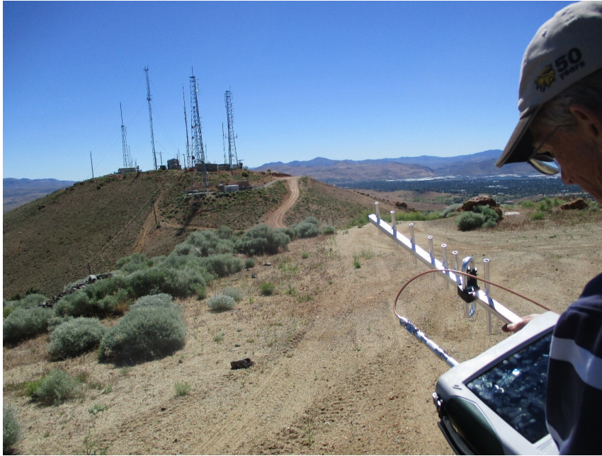
Figure 11. Revalidating the source of the interference from a distant location.
