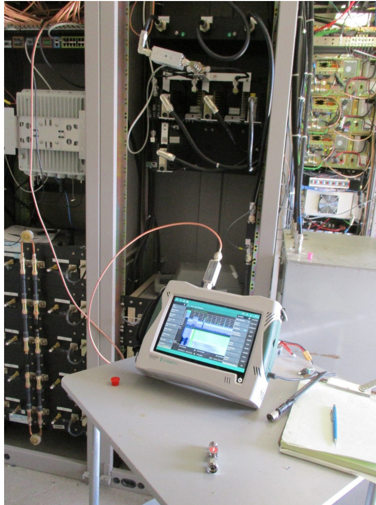
Figure 4. The Field Master Pro MS2090A connected to the P25 system receiver RF test port with the high-pass filter in line.
