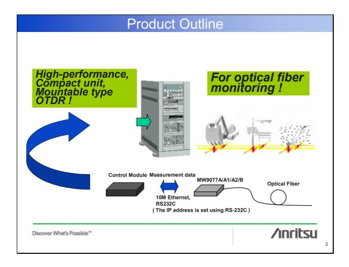
I will first provide an outline of the MW9077A/A1/A2/B OTDR module.
