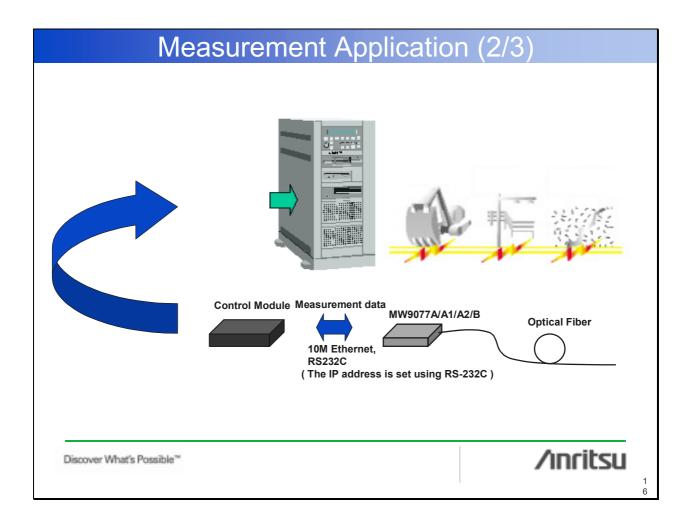
This slide shows an example of an OTDR measurement environment.
