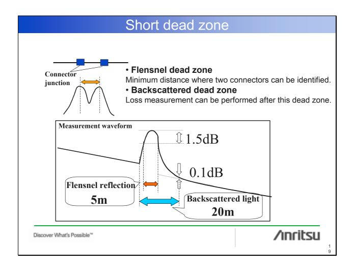
The dead zone values of the MW9077 series are 5 m (Fresnel reflection) and 20 m (backscattered light).
