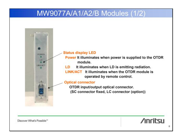
This slide shows the front of the MW9077A/A1/A2/B OTDR module.
