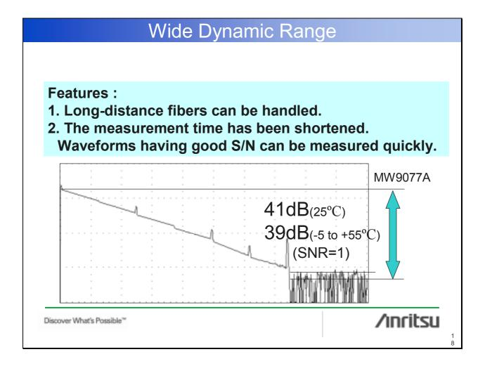
One of the essential parameters when performing OTDR measurements is the dynamic range.
