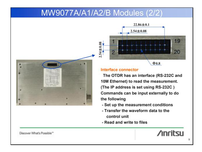
The MW9077A/A1/A2/B has the interface connector shown in the figure. All commands used for setting up the measurement conditions, starting and stopping measurement, and so on are executed through these interfaces. Both the 10M Ethernet and RS-232C interfaces can be used. (The IP address is set using RS-232C.) Commands can be input externally to do the following:
