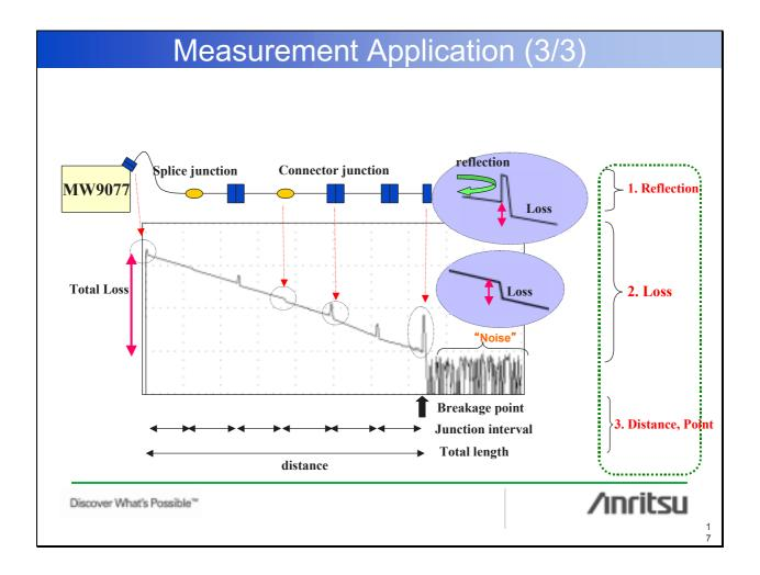
The MW9077A/A1/A2/B OTDR module measures events automatically (locations of connection points, connection loss, reflection amount, and total fiber connection loss). (Regarding automatic detection, please note that, depending on the measurement environment, not all of the points may be accurately detectable.)
