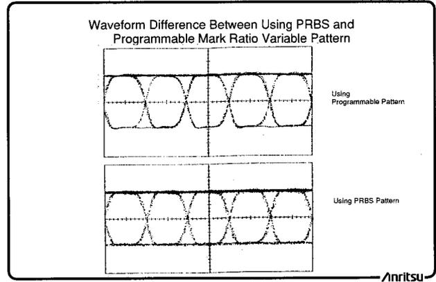
In Anritsu's MP1763C, there are even two methods built-in for generating variable mark ratio patterns using PRBS.
