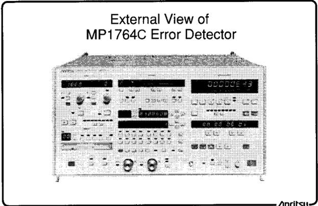
This photograph shows the error detector input section. The delay and threshold level can be set with high resolution. The delay can be set in 1 ps steps. The threshold level of Anritsu error detectors can be varied in 1 mv steps. The resolution is sufficient for detecting the minimum error generation point. The threshold level and delay can be set automatically to the best point using the Auto-Search function. Also, eye margin measurement is possible.
