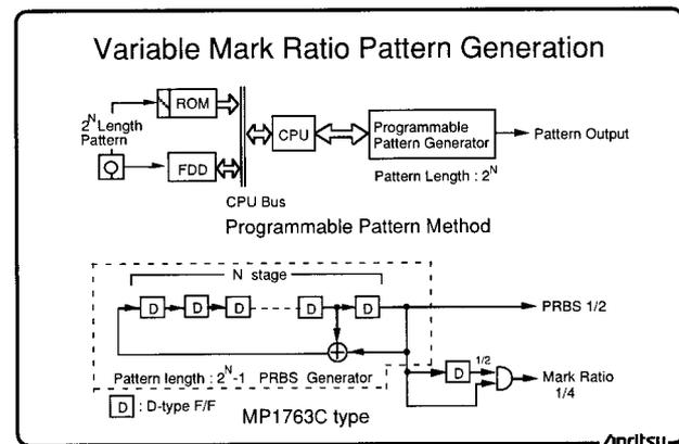
Also, the measurement pattern must have a secure randomness for the pattern cycle. By using the programmable pattern method, the cycle becomes  $2^N$  as already described before, but the  $2^N$  value has a lot of factors. What is the meaning of this? This can be clarified from the waveforms. The upper one has a pattern equivalent to the  $2^{10}$  cycle variable mark ratio pattern which was loaded from firmware.
