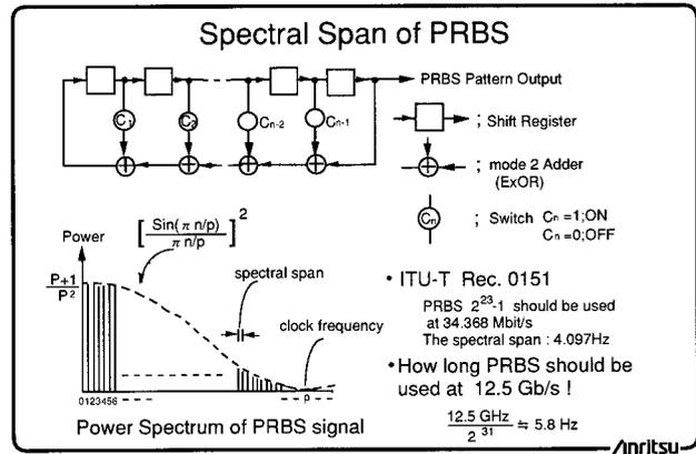
The variable mark ratio pattern generation is an extremely important function of a PPG. This BERTS family has the capability of creating a PRBS pattern with variable mark ratio. there are two generation method of variable mark ratio pattern one providing with programmable patterns and the other using PRBS pattern.
