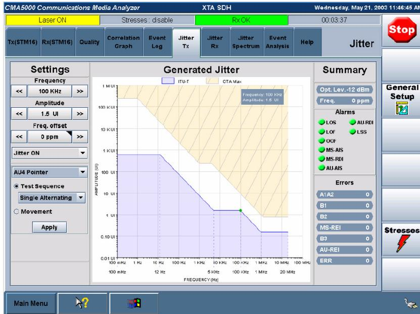
Figure 11. Jitter generation configuration with CMA5000 XTA
