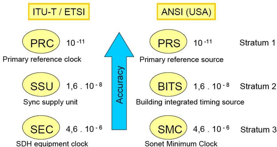
Figure 2. Two clocks hierarchies in the synchronous world
