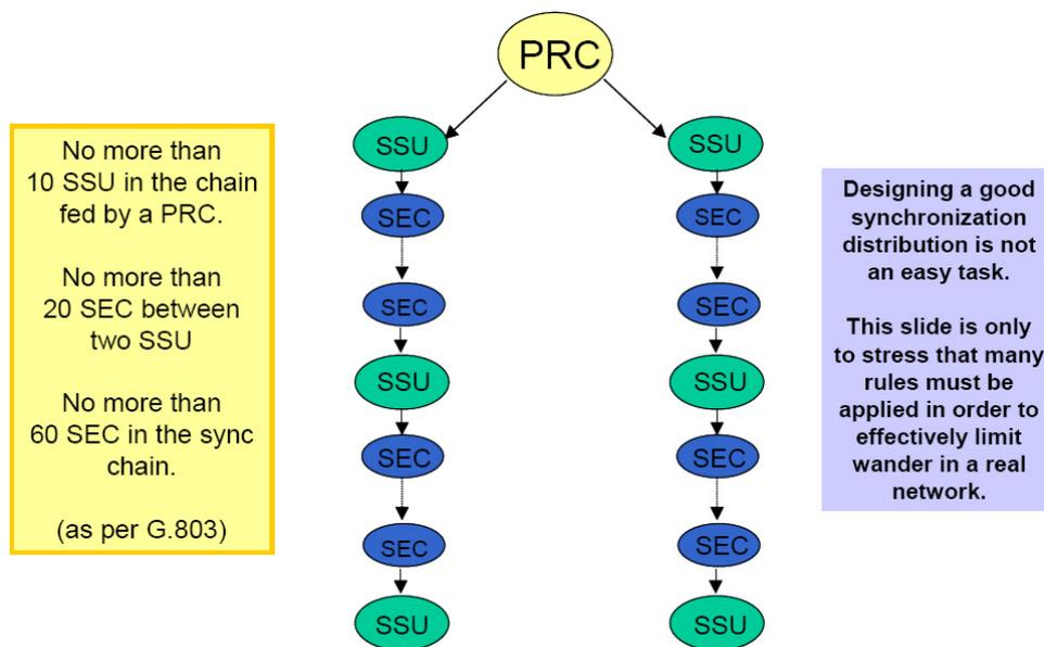
Figure 3. Synchronization distribution in SDH terms (Master – Slave type)
