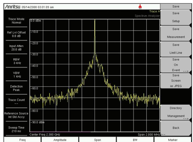
Figure 2: CW signal with phase noise
