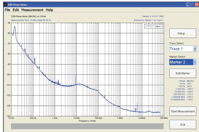
Figure 3: Example phase noise plot with jitter measurement from 10 kHz to 5 MHz offset; markers delimit the frequency offset range for the jitter measurement.
