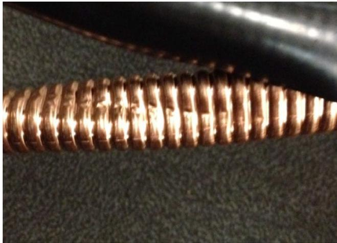
Figure 9. Cable Damage
