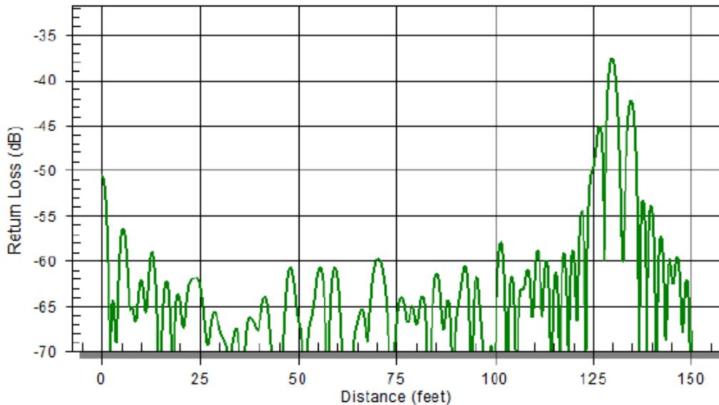
Figure 3. Typical Distance-to-Fault Loss Sweep
