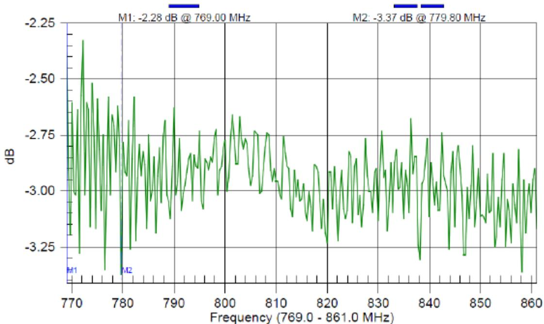
Figure 2. Typical Return Loss Sweep
