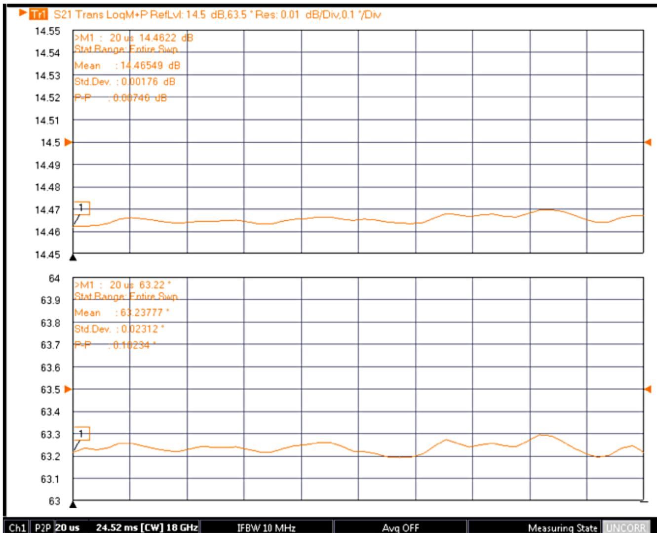
**Figure 3.** An example classical P2P measurement is shown here where one measurement is performed per pulse. If the behavior in a particular part of a pulse is all that is of interest, this can be an easier way to visualize longer-time-scale distortions.
