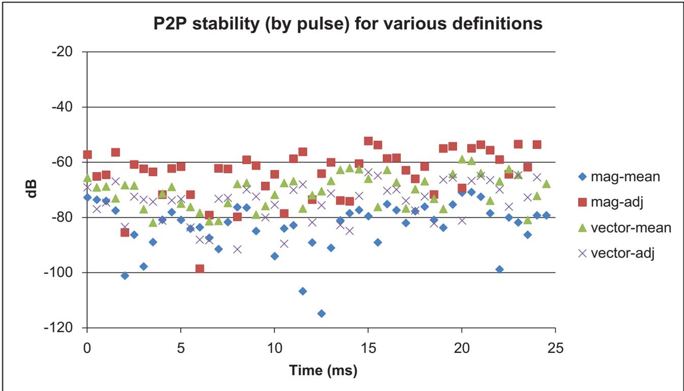
**Figure 4.** Some of the pulse-to-pulse stability metrics are plotted here for a set of example data. The individual terms in the summations presented in the text are plotted to help show the differences more clearly.
