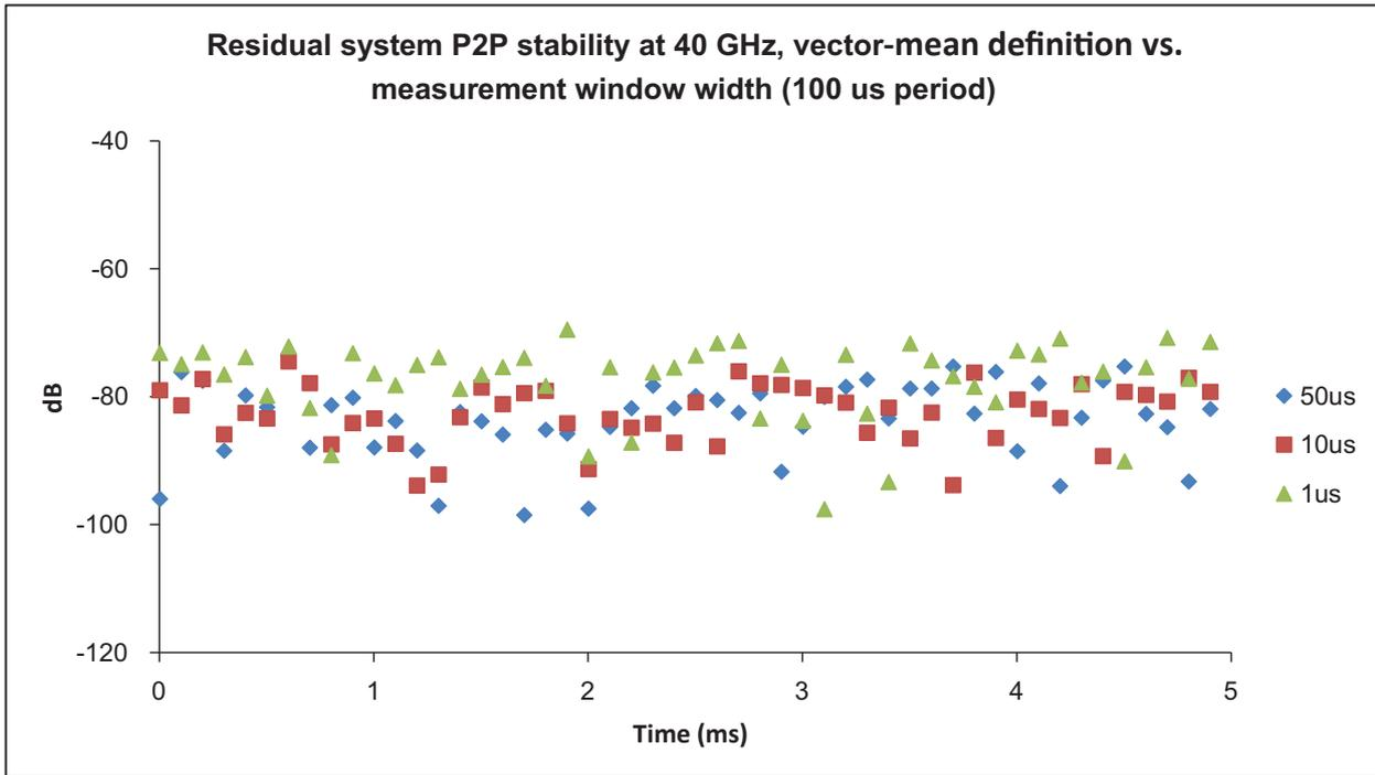
**Figure 6.** Example residual P2P stabilities for the MS464XB at 40 GHz for a variety of measurement window widths are plotted here. This value would apply equally for a start-up transient kind of measurement or a quasi-steady-state measurement
