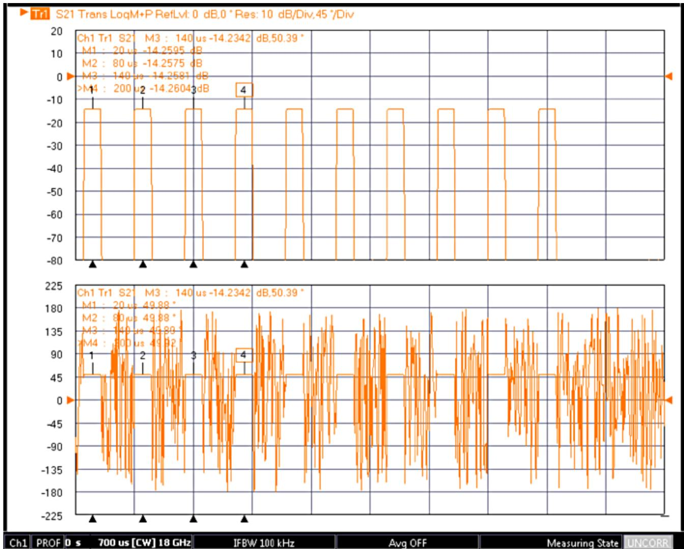
Figure 2. An example profiling-like pulse-to-pulse measurement is shown here. The resolution can be very high (to 2.5ns with the MS464XB) and allow detailed analysis.
