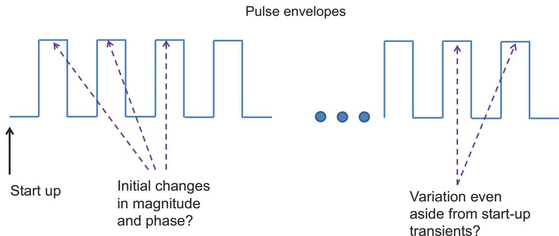
**Figure 1.** The pulse-to-pulse (P2P) measurement situation and the distinction between start-up-related and quasi-steady-state measurements are shown here.
