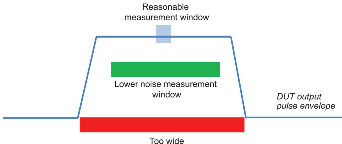
**Figure 5.** While many measurement window widths can be used, optimizing the width (if possible for a given application) can result in improved noise performance.
