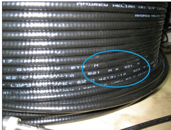
The Commscope LDF-2 cable was marked every meter.
