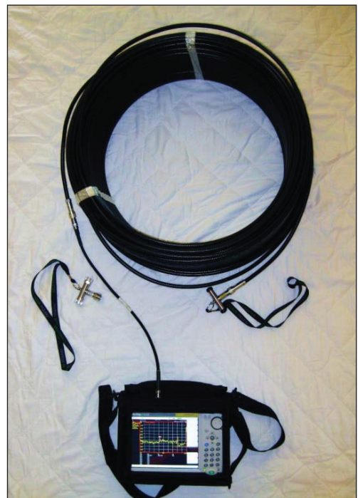
A 605 ft length of LDF-2 with N-M connectors installed, S412E, 15NNF50 test port cable, OSLN50
