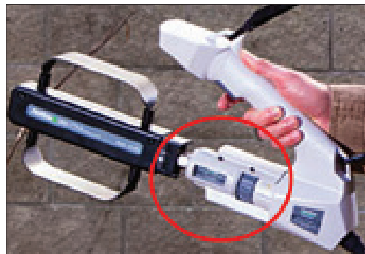
Figure 6. Pre-filter (bandpass filter) in place between an antenna and the MA2700A
