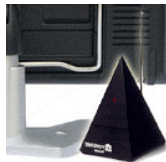
Figure 10. A broken RF TV remote can cause interference
