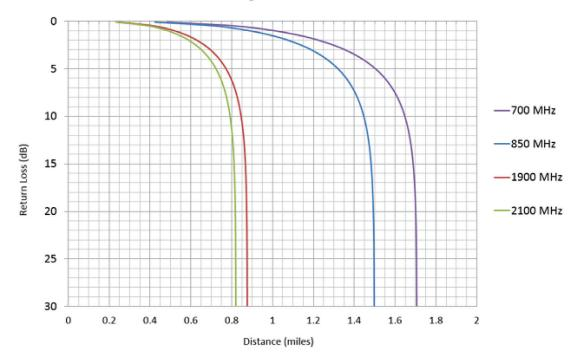
Looking at specific examples, the change in coverage distance can be evaluated for a return loss improvement from 15 dB to 18 dB (3 dB improvement) and from 17 dB to 18 dB (1 dB improvement) as shown in Table 2 and Table 3. As can be seen, the coverage distance is improved, but only slightly.
