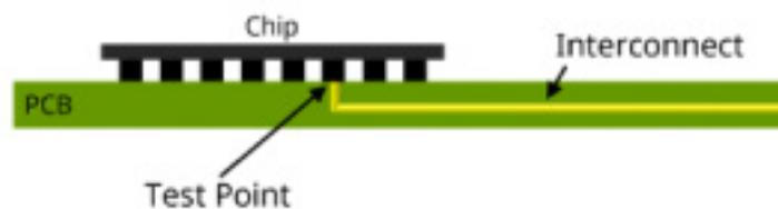
Figure 23. The test fixture must be de-embedded from measurements so that we can evaluate the signal at the test point.
