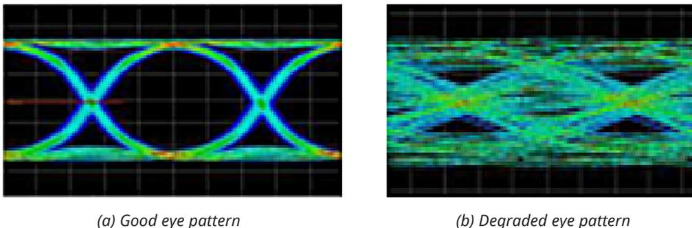
Figure 2. Eye diagrams show amplitude and time distortions which allow signal impairments in the physical layer to be easily seen.
