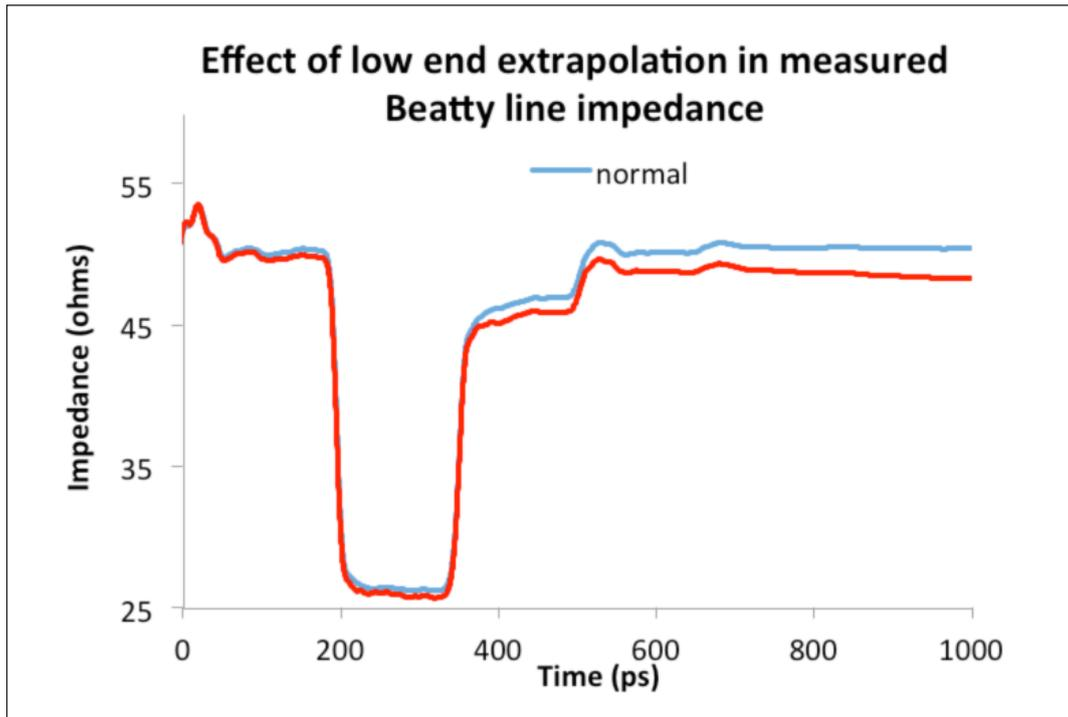
(c) Effect of poor low frequency accuracy
