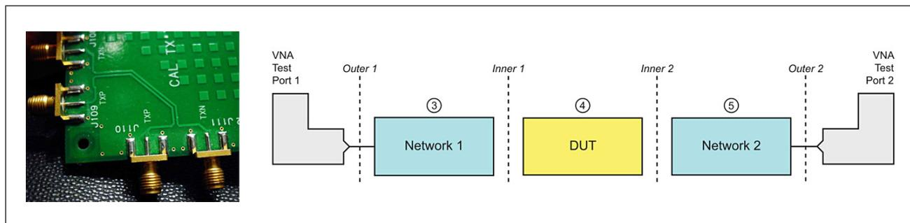
Figure 24. Embedding techniques allow you to insert the effects of network elements by using the S-Parameters of one or more connectors or fixtures on one or both test ports.
