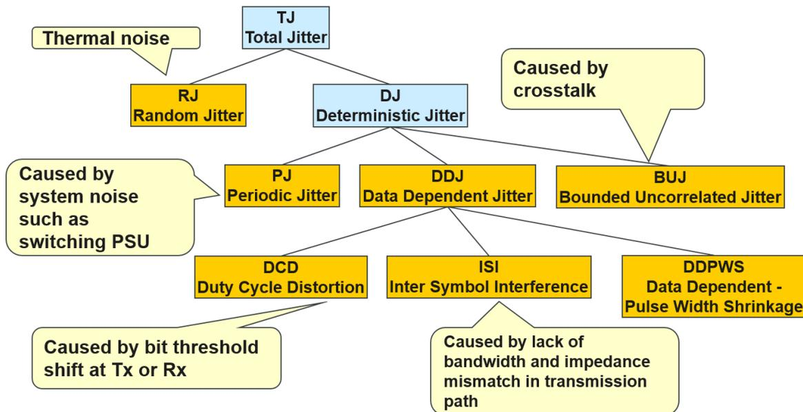
Figure 12. Total jitter is caused by a wide variety of factors.
