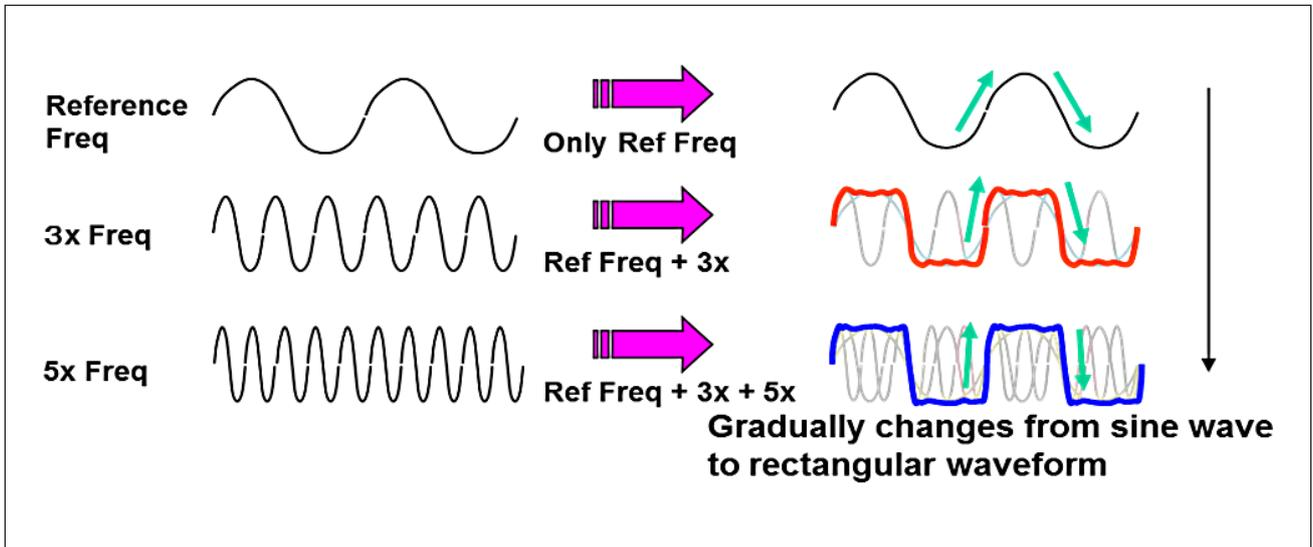
Figure 3. A square wave is composed of an infinite number of odd harmonics.
