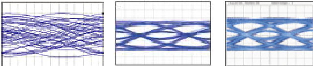
(a) 0.5 dB insertion loss error at 10 MHz
