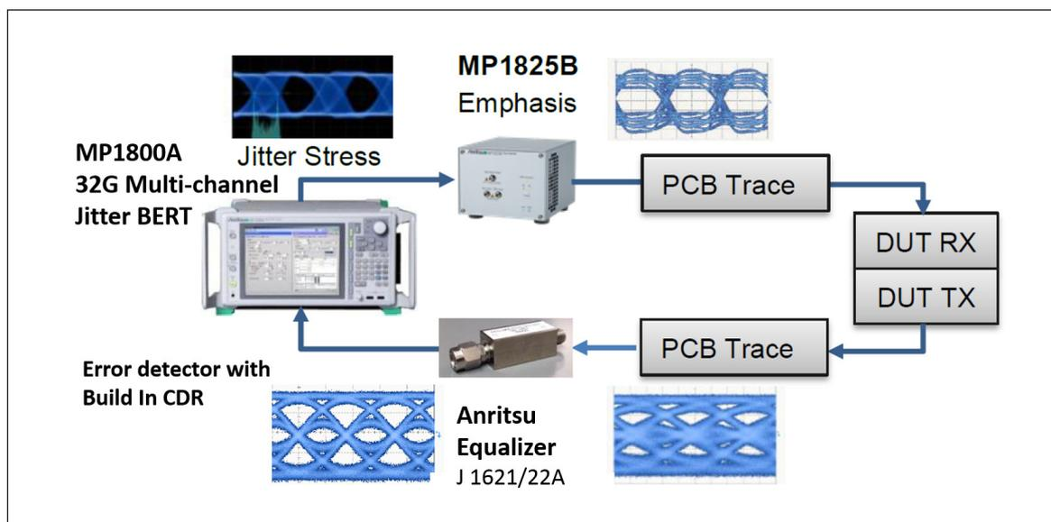
Figure 14. BERTs are excellent at determining if there are any issues with jitter, the bit error rate, and eye openings.
