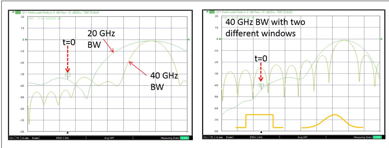
Figure 22. Basic causality is always impacted by available finite bandwidth. VNAs offer multiple time domain windowing functions (right), which can also have a major effect on the measured result. Note the signal levels for  $t < 0$ .
