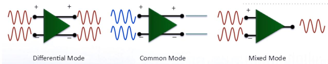
Figure 9. Differential lines provide rejection of external fields, have minimal radiation and are commonly used to interconnect devices.
