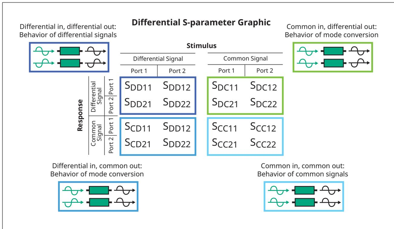
Figure 11. Sixteen parameters are required to describe the various combinations of differential and common mode signals.
