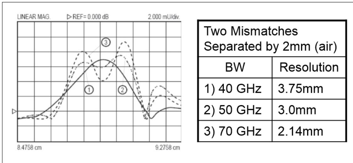
Figure 19. Getting the best time domain resolution requires the most data points, narrowest frequency step size, and widest possible frequency bandwidth.
