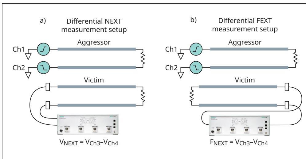
Figure 7. Closely spaced parallel micro-strip lines can couple signals unintentionally.
