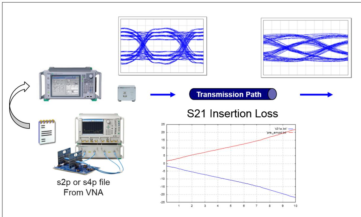
Figure 5. Test setup block diagram for determining the ideal emphasis setting for a given transmission line [Blue trace s31a.txt is the measured insertion loss, Red trace pre\_ampd.txt is the corresponding emphasis].
