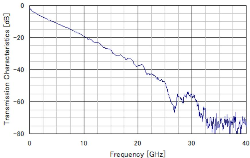
Figure 4. Attenuation or loss increases with frequency and may negatively impact the eye opening.
