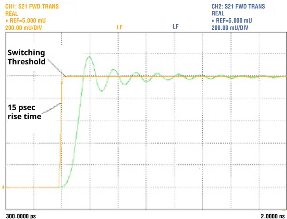
Figure 13. The result of SWR on a pulsed signal is ripple which can cause false triggers.
