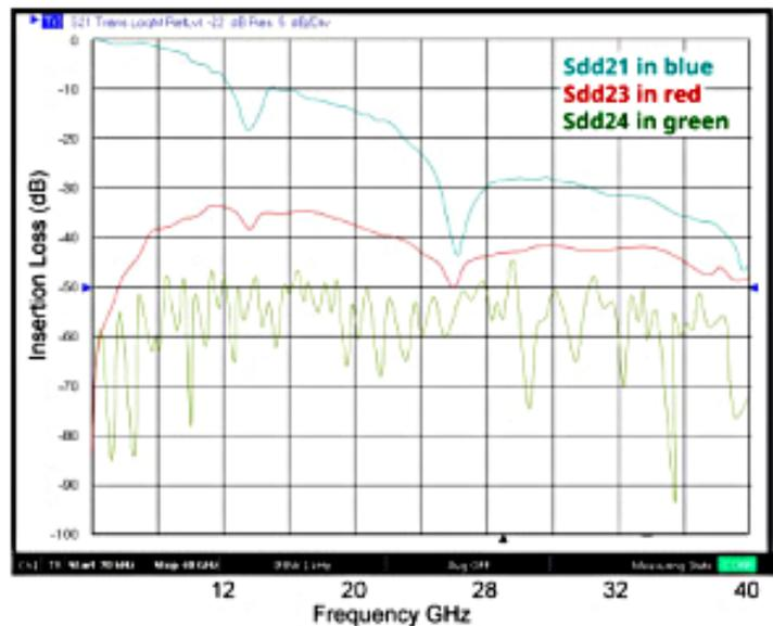
Figure 8. Insertion loss, NEXT and FEXT for a differential channel in a two channel differential system. Sdd21 (insertion loss), Sdd24 (NEXT), and Sdd23 (FEXT).
