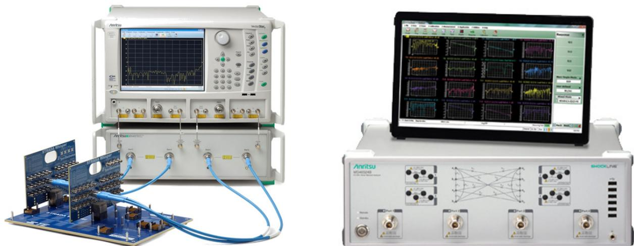
Figure 15. VNAs are useful for determining the cause of a signal integrity issue.
