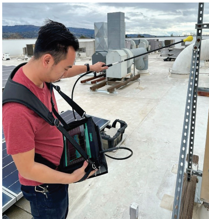
PIM Hunting with Field Master MS2080A and 2000-1884-R PIM Hunter Probe
