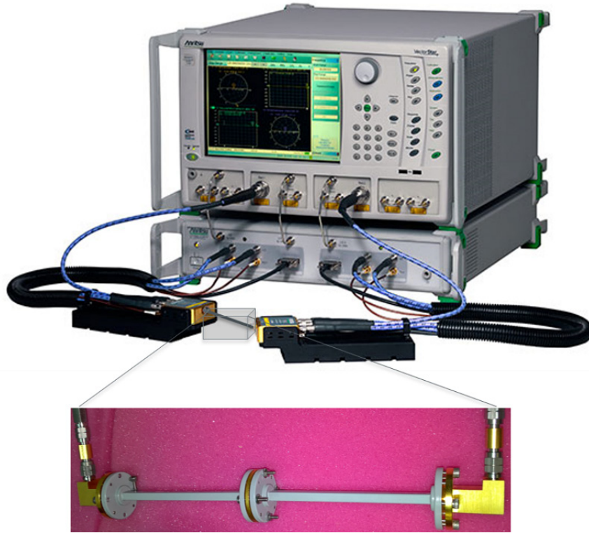
Figure 2. Transmission line setup for broadband materials measurements. The setup is composed of an Anritsu VectorStar™ ME7838E VNA with 70 kHz to 110 GHz (1 mm coaxial output) full sweep capability and a set of waveguide components covering the wideband range. At the bottom, a zoom of a WR-19 waveguide transmission line is shown, with the MUT located at the central junction.
