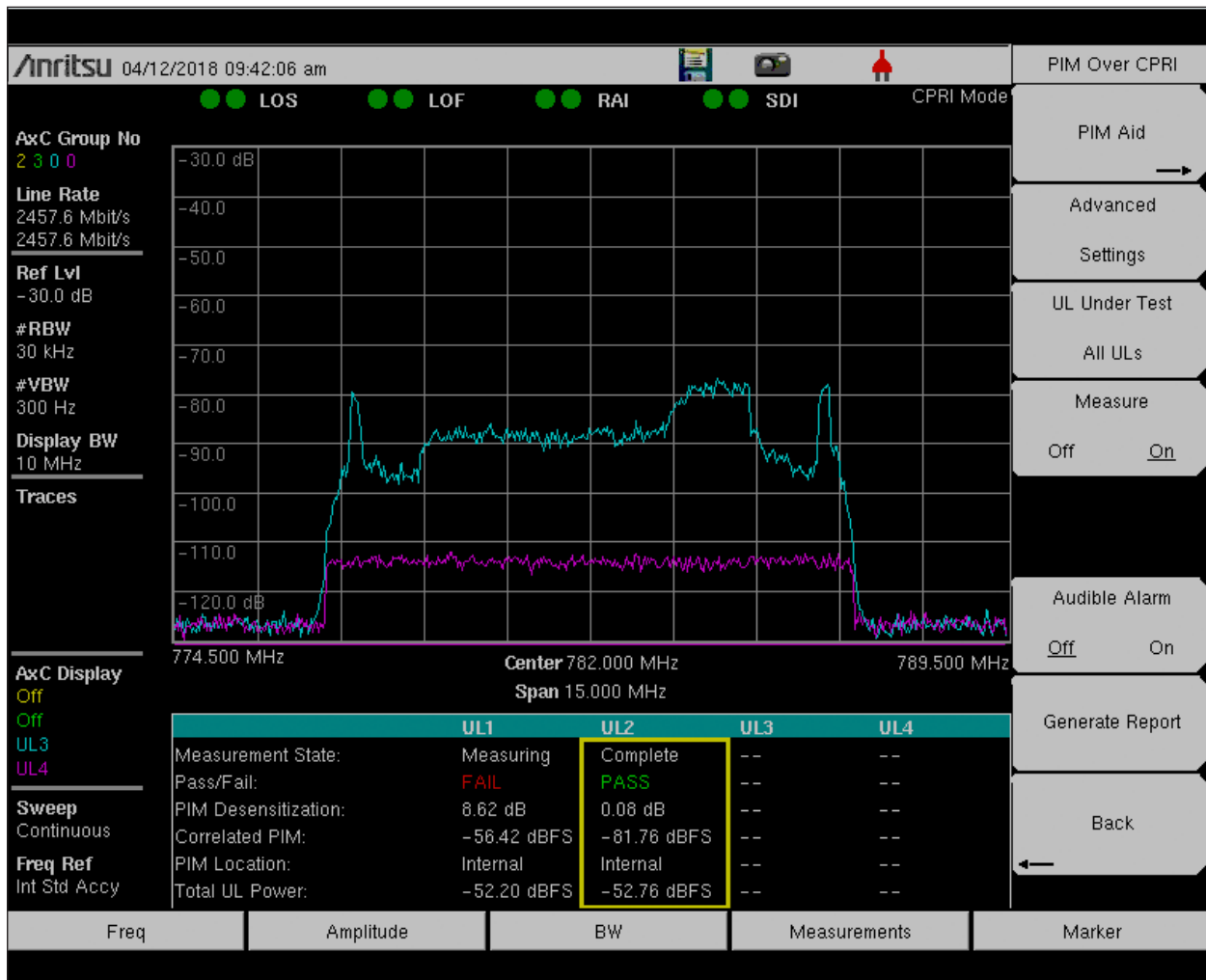
Figure 4. Example of Measurement, active UL2 with NO PIM present
