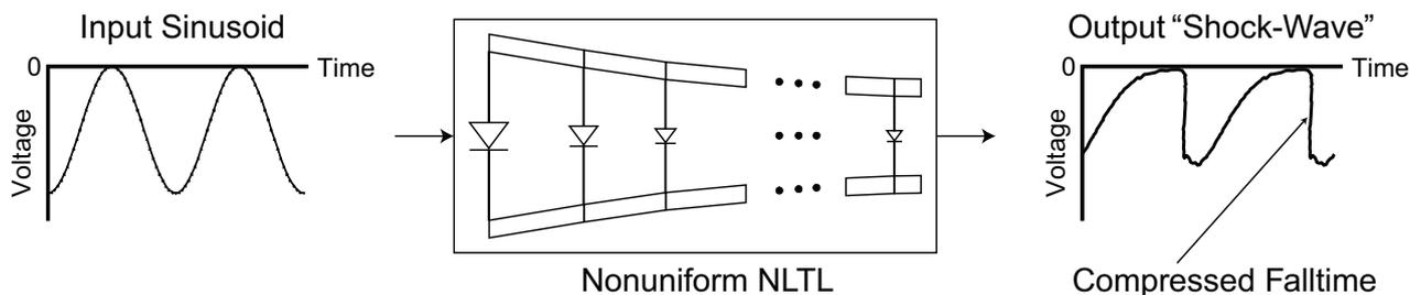
Figure 2. The enhanced fall time compression and use of a differentiator circuit (step differentiation) transforms a continuous wave signal into a train of pulses used for sampler gating.
