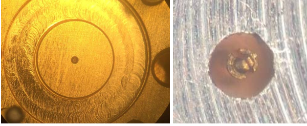
Fig. 3. The female side of the broadband interface is shown on the left (module side) and the male pin (used on the probe) is shown on the right. The outer conductor diameter is 0.6 mm.
