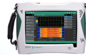
MS2090A Field Master Pro 9kHz – 54GHz
