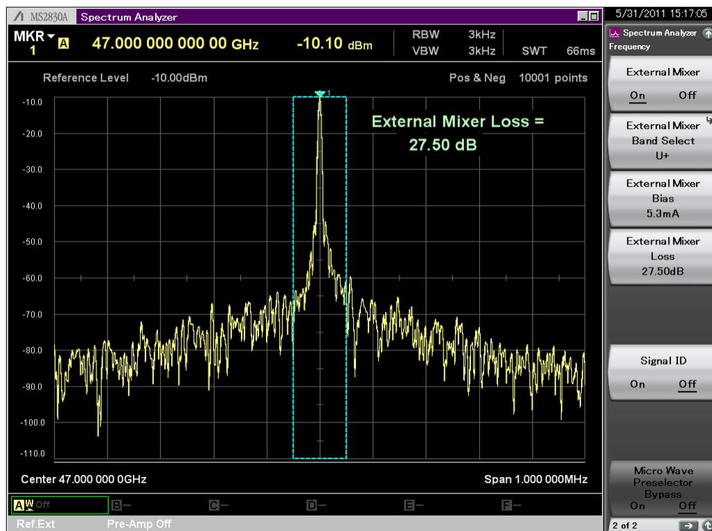
図5. External Mixer Bias, External Mixer Lossの設定例
