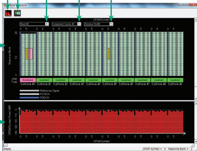
Frame Structure画面 (LTE-Advanced)
