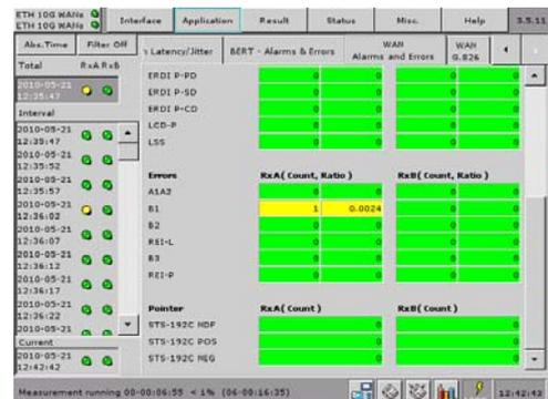
Fig. 16 Statistics for analysis of the transmission-error performance.
