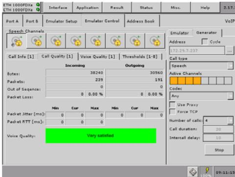
Fig. 13 A total of 8 VoIP calls can be generated through the CMA 3000's two Ethernet test ports. The voice quality evaluation is presented for one call if the Voice Quality Measurement option is installed.
