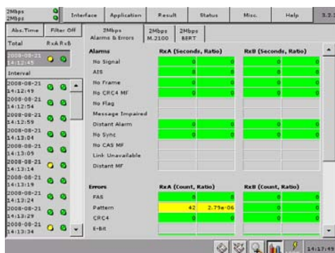
Figure 6 CMA 3000 gives comprehensive statistics on alarms and errors.
