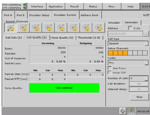
Fig. 13 A total of 8 VoIP calls can be generated through the CMA 3000 Ethernet's two test ports. The voice quality evaluation is presented for one call if the Voice Quality Measurement option is installed.
