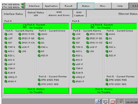
Fig. 15 A quick overview of the alarm and error status on the line.
