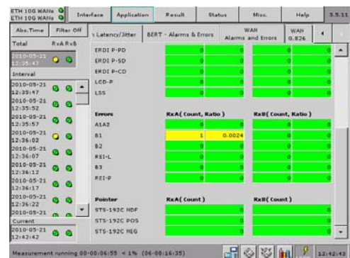
Fig. 16 Statistics for analysis of the transmission-error performance.
