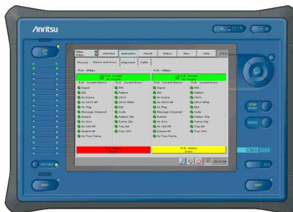
Fig.2: With FrontSim you can operate a remote CMA 3000 from a PC.
