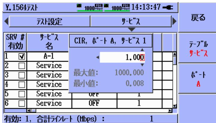
This screenshot shows the same 'Y.1564テスト' interface as above, but the 'CIR (Mbps)' cell for service 'A-1' is now open in an edit dialog. The dialog displays the current value '1.000', with '最大値: 1000.000' (Maximum: 1000.000) and '最小値: 0.008' (Minimum: 0.008). The 'CIR' column header is also highlighted with a red border. The 'CIR, ポートA, サービス 1' label is visible above the edit field.
