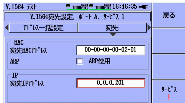
The screenshot shows the 'Y.1564宛先設定' (Y.1564 Destination Setting) screen. It includes fields for MAC (宛先MACアドレス: 00-00-00-00-02-01, ARP: ARP使用) and IP (宛先IPアドレス: 0.0.0.201). The '宛先IPアドレス' field is highlighted with a red border. To the right, there are buttons for 'アーフル' (Arful), 'ポート' (Port), and 'サービス 1'.
