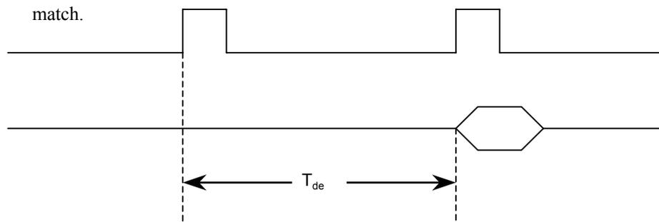
**T<sub>de</sub>**: The external trigger signal is the delay time for burst signal output, the time from the trigger signal to the rising edge of the first slot of the frame.
