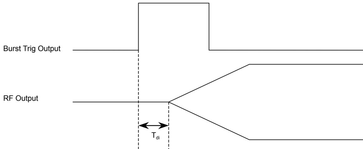
$T_{di}$ : The internal trigger signal is the delay time for burst signal output, the time from the trigger signal to the rising edge of the first slot of the frame.
