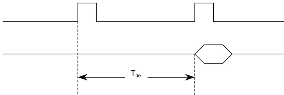
$T_{de}$ : Represents the delay time when a burst wave is output using the external trigger signal, which corresponds to the time from trigger signal until the start up of the first slot in the frame.
