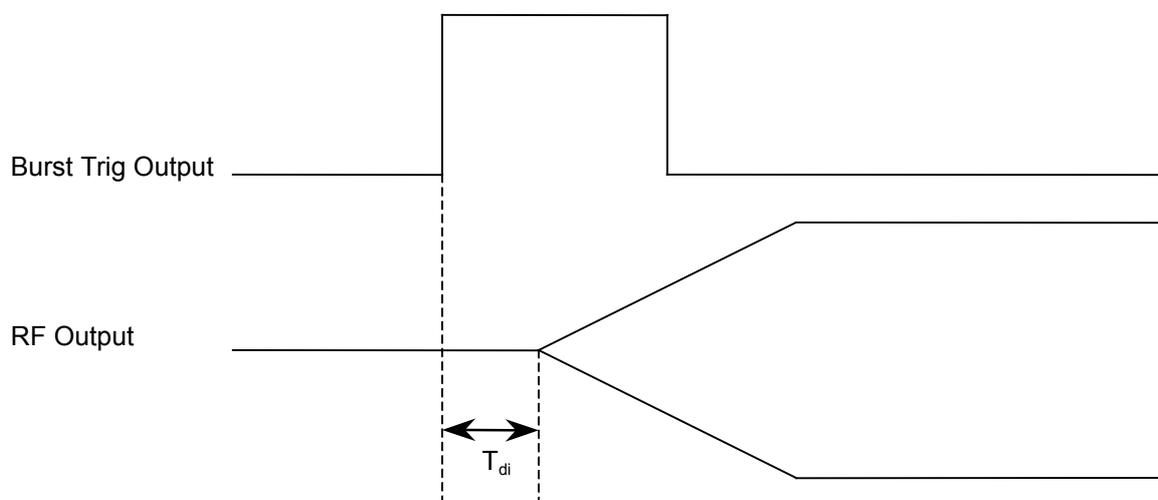
$T_{di}$ : Represents the delay time when a burst wave is output using the internal trigger signal, which corresponds to the time from trigger signal until the start up of the first slot in the frame.
