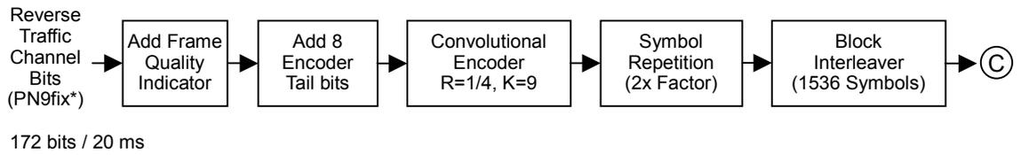
Fig. 3-3 Device Test Signal–Block diagram of 1xRTTTrc3(1)\_RVS (Part1/2)
