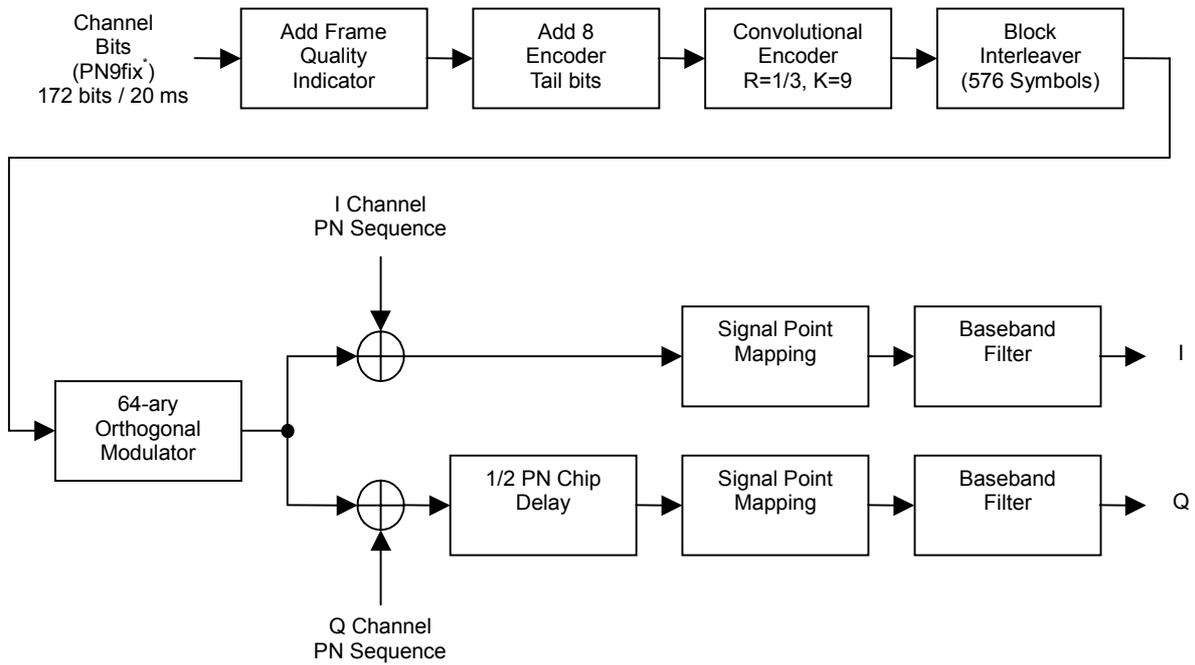
Fig. 3-1 Device Test Signal–Block diagram of 1xRTTtrc1\_RVS
