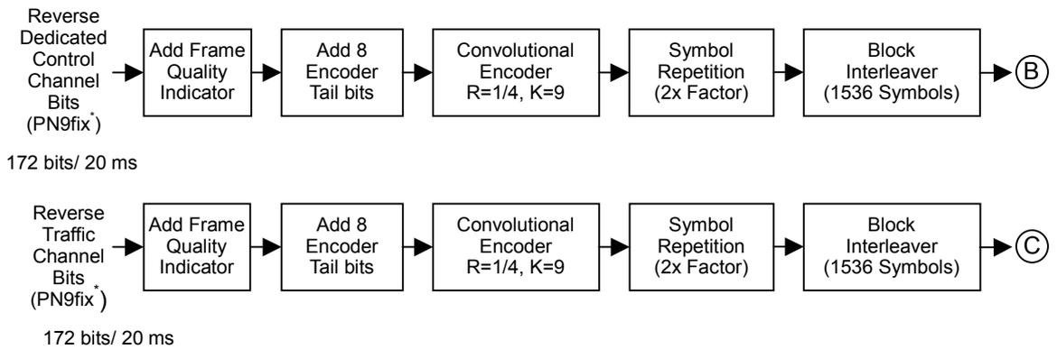
Fig. 3-7 Device Test Signal-Block diagram of 1xRTTtrc3(3)\_RVS (Part1/2)
