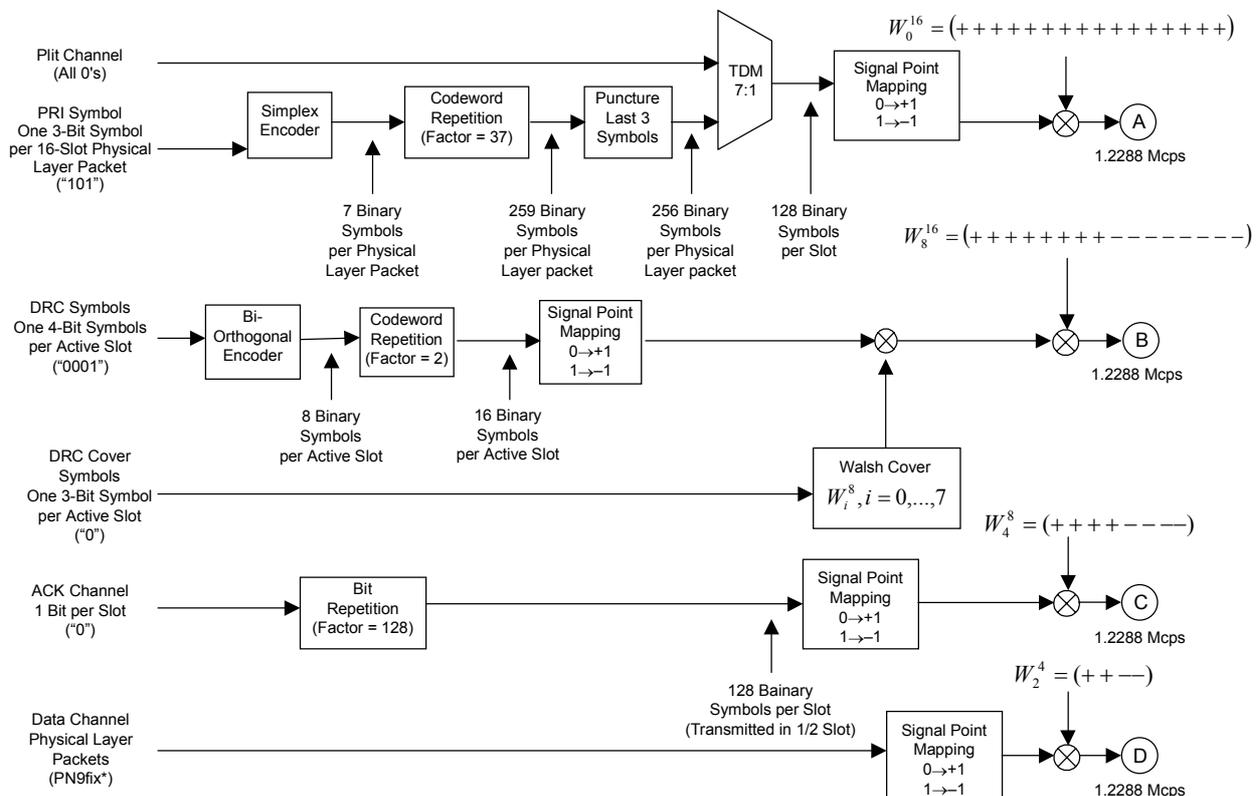
Fig. 3-14 Device Test Signal-Block diagram of 1xEV-DO\_RVS (Part1/2)
