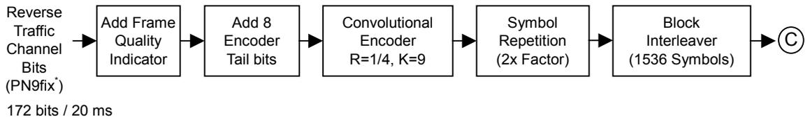
Fig. 3-5 Device Test Signal–Block diagram of 1xRTTTrc3(2)\_RVS (Part1/2)
