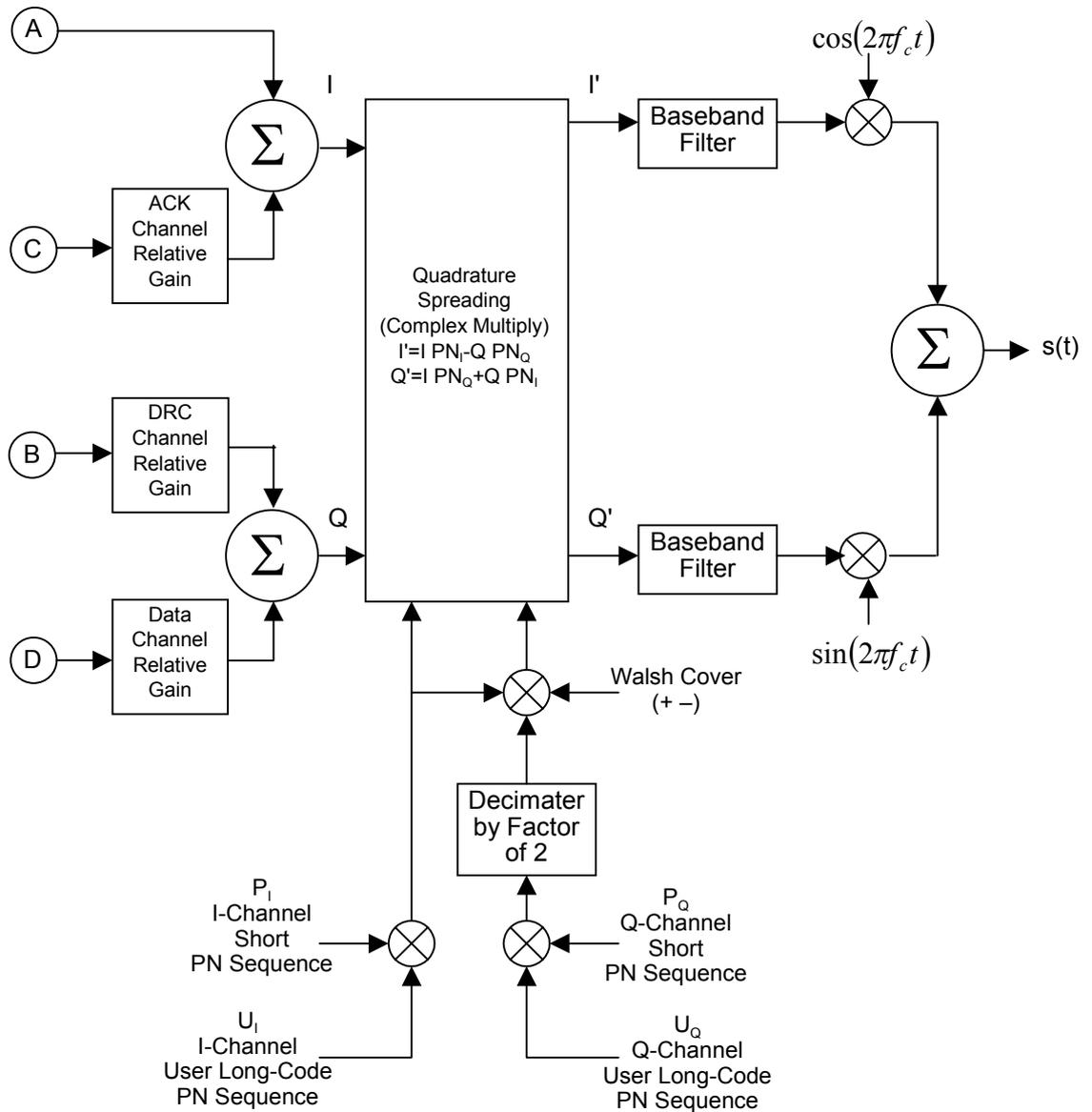
Fig. 3-15 Device Test Signal–Block diagram of 1xEV-DO\_RVS (Part2/2)
