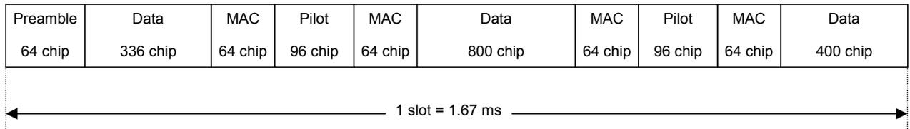
Fig. 3-13 Device Test Signal–Block diagram of 1xEV-DO\_FWD (Part2/2)
