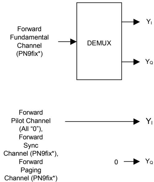
Fig. 3-10 Device Test Signal–Block diagram of 1xRTTrc3-5\_FWD (Part1/2)
