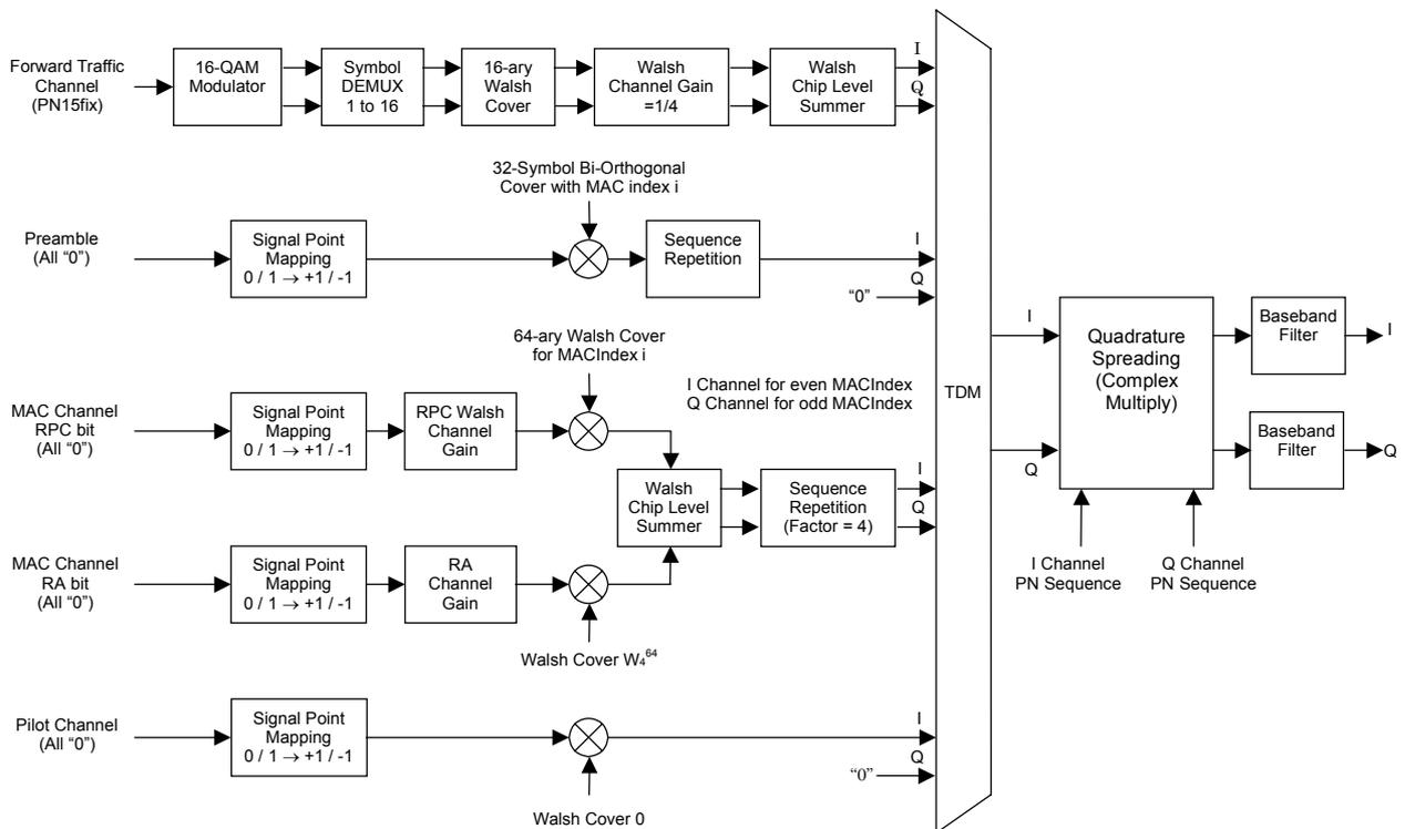
Fig. 3-12 Device Test Signal-Block diagram of 1xEV-DO\_FWD (Part1/2)
