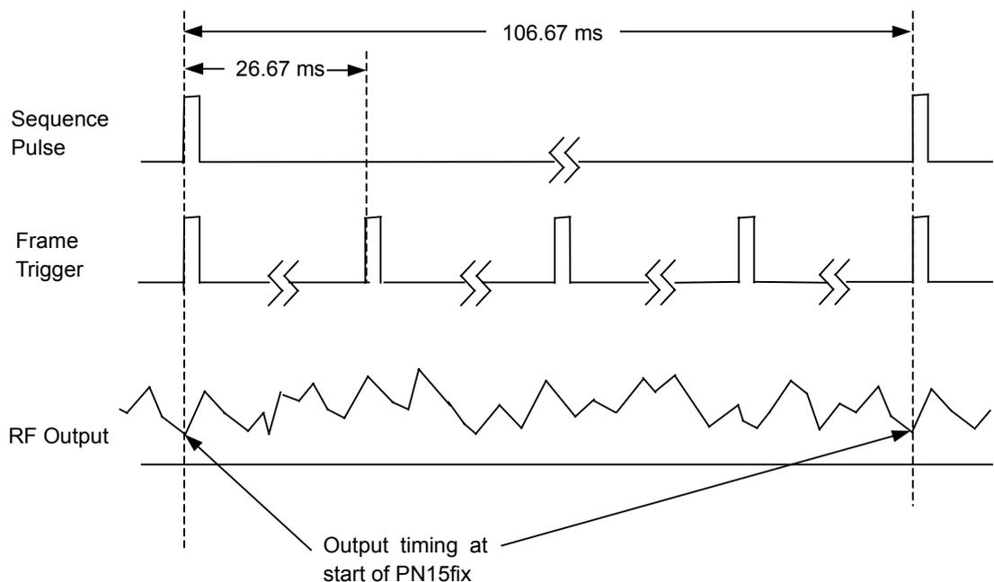
Figure 3-11 Trigger Timing for Forward (excluding Idle Slot)
