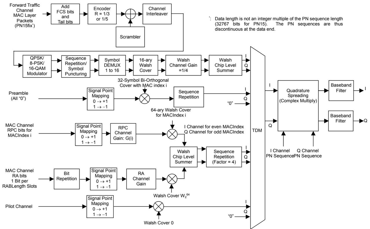
Figure 3-2 1xEV-DO Forward Block Diagram
