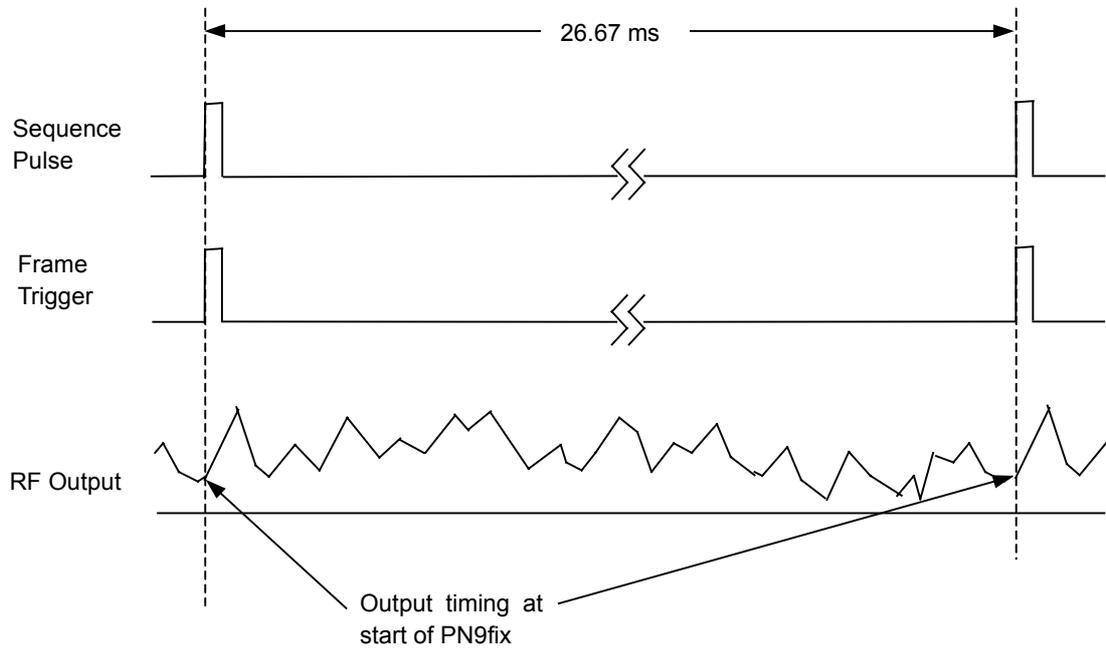
Figure 3-12 Reverse Trigger Timing
