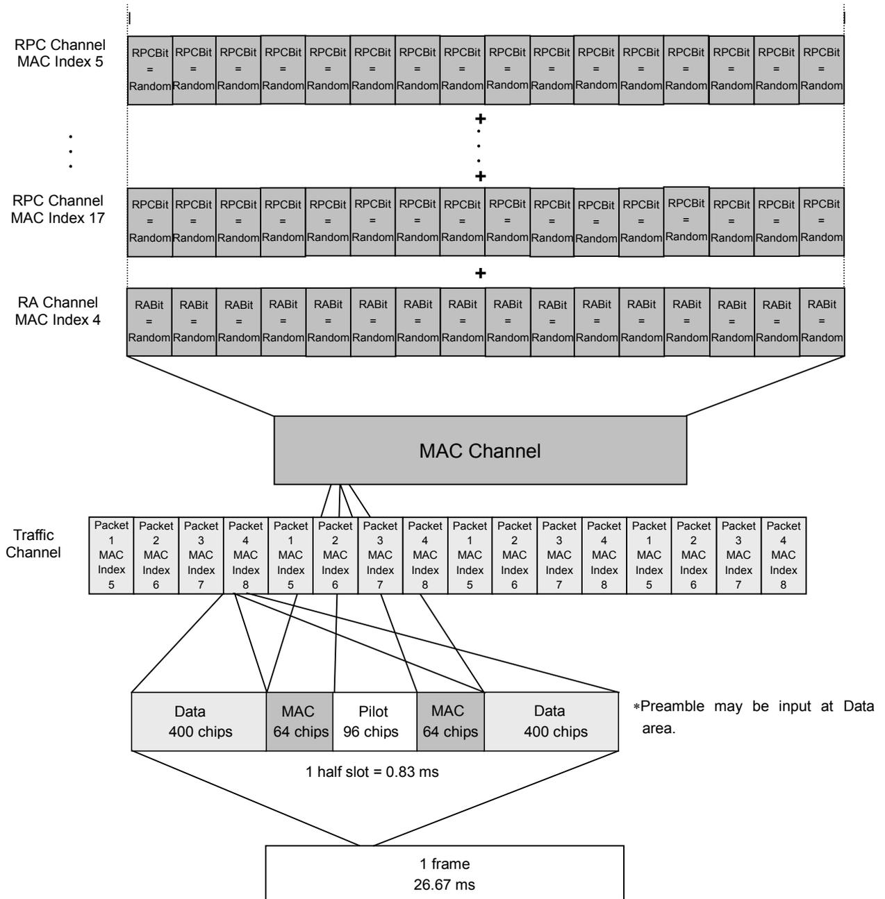
Figure 3-5 Multiplexing of each Channel
