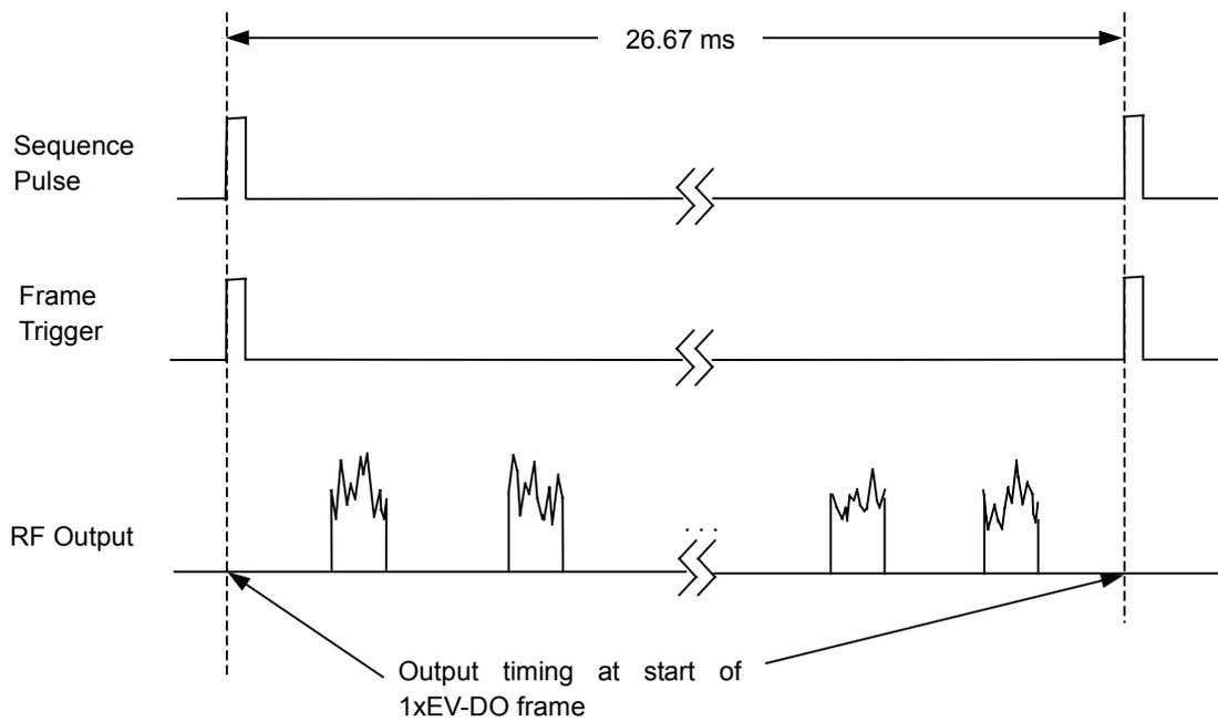
Figure 3-13 Trigger Timing for Forward Idle Slot
