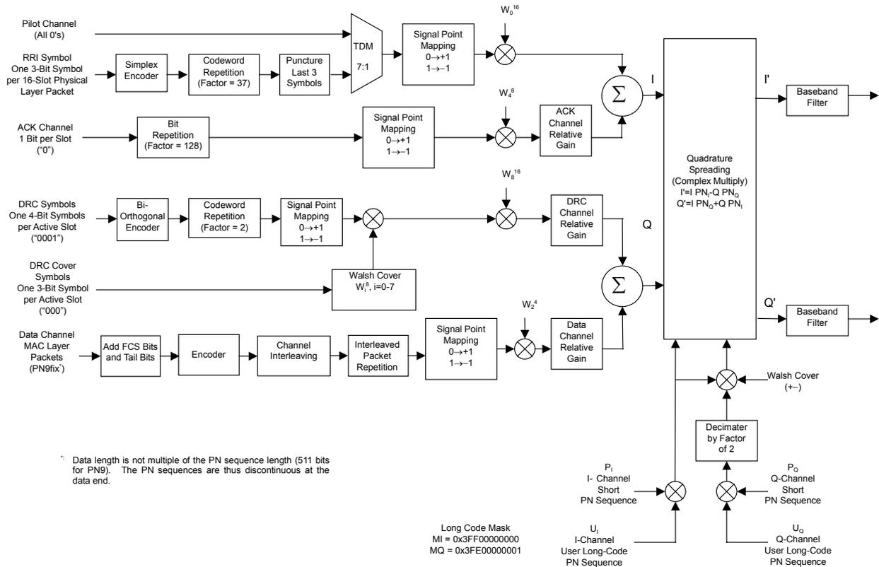
Figure 3-7 1xEV-DO Reverse – Block Diagram
