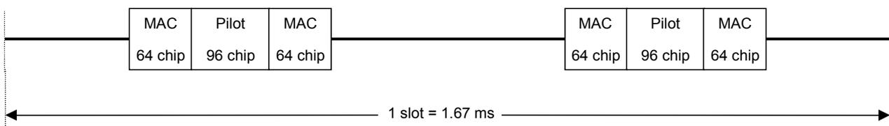
Figure 3-9 1xEV-DO Forward Idle Slot Format
