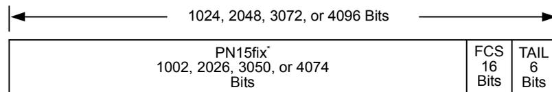
**Figure 3-1 Forward Packet Format**
