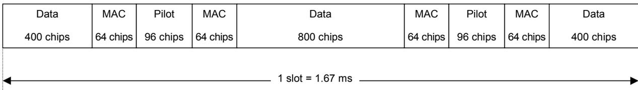
Figure 3-3 Slot Format of 1xEV-DO Forward (without idle slot)
