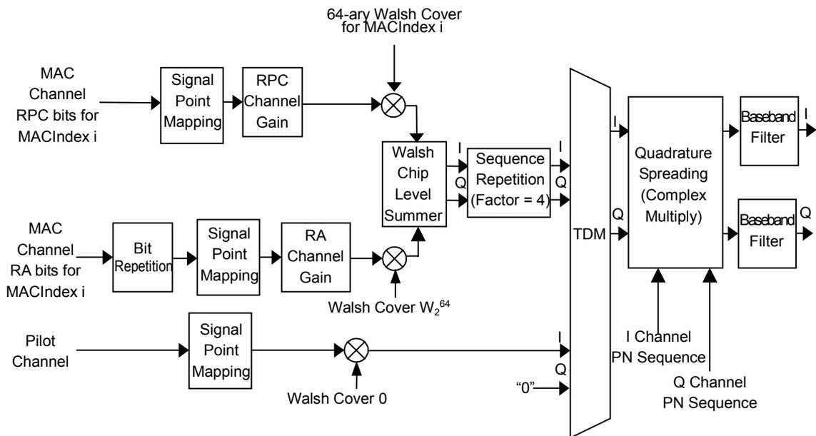
Figure 3-8 Forward Idle Slot – Block Diagram
