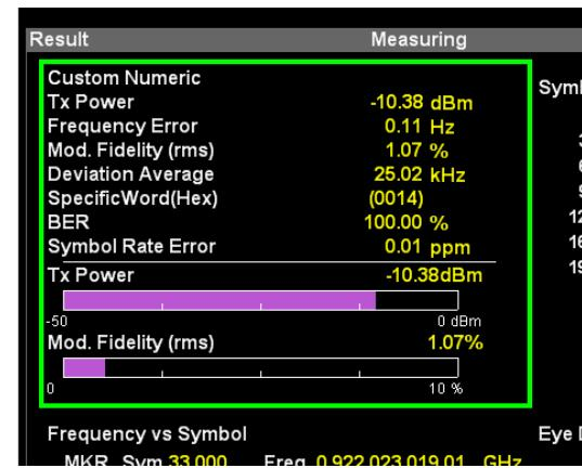
Numeric and graphical results can be checked simultaneously on 4 sub-screens by displaying any item from the many numeric results on the Numeric screen. Moreover, difficult-to-evaluate numeric values can be evaluated intuitively from bar graphs.
