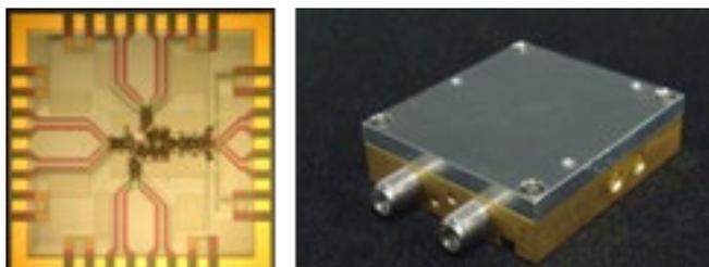
Figure 4: InP HBT MMIC and Hybrid Module Appearance
