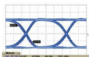
Figure 2: 56 Gbit/s NRZ Waveform    Figure 3: 28 Gbit/s NRZ Waveform
