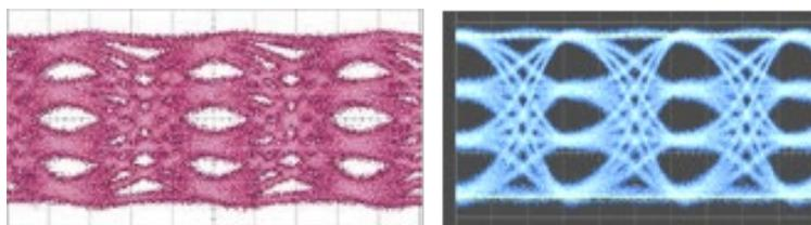
Figure 8: 56 Gbaud PAM4 Waveform Figure 9: 28 Gbaud PAM4 Waveform
