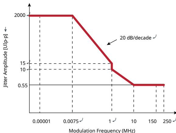
Figure 10: MP1800A Series 64 Gbit/s BERT SJ Max. Modulation
