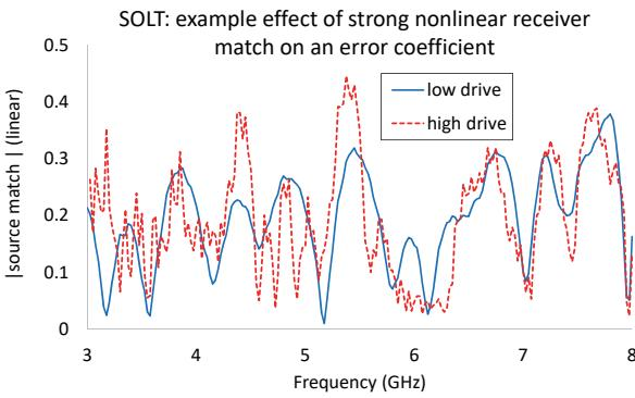
Figure 6 Example effect of LNA nonlinear match on a short-open-load calibration error term.
