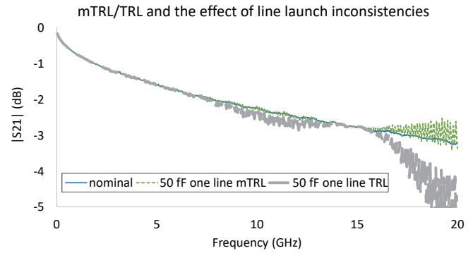
Figure 10 The effect of a changing launch parasitic capacitance on the calibrated insertion loss measurement of a DUT is shown here. When one line is deviant, mTRL can be less sensitive than TRL.
