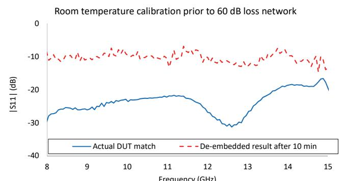
Figure 2 De-embedding high loss networks can result in high sensitivities. The lower repeatabilities in cryogenic measurements can lead to poor stability when de-embedding is done classically.
