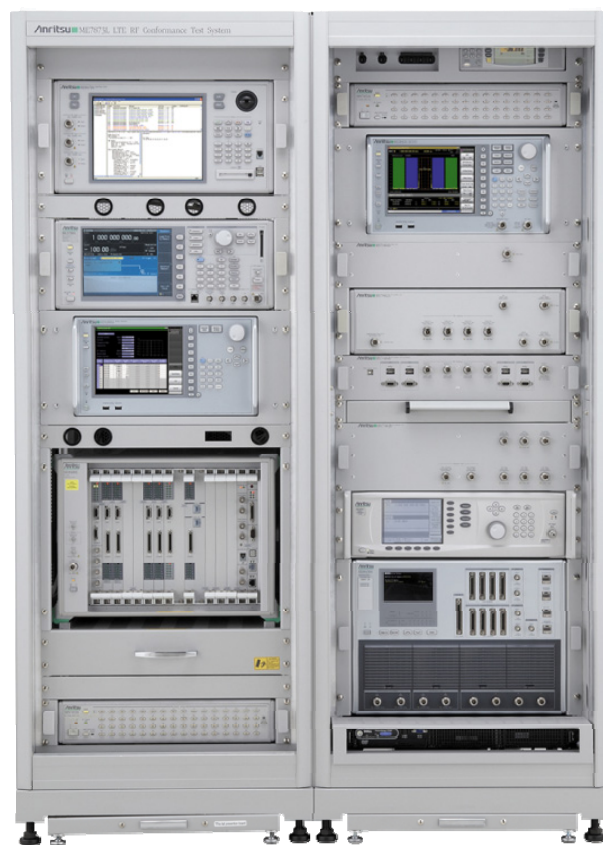
Figure 1 ME7873L RF Conformance Test System
