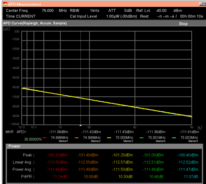
Figure 11 32000-ch APD Spectrum (floor noise)
