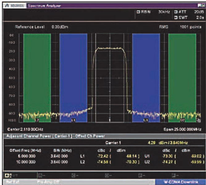
Figure 4 W-CDMA Measurement Example (Test Model1_64DPCH)
