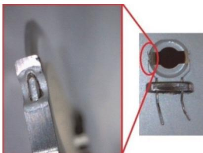
Figure 13 Damaged Crystal Resonator
