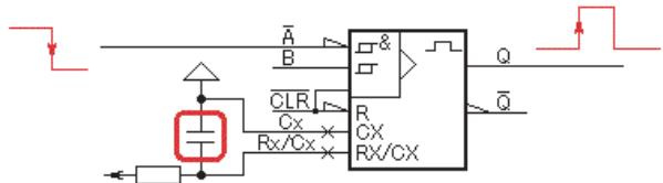
Figure 7 Monostable Multivibrator IC
