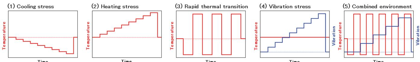
Figure 1 HALT Procedure
