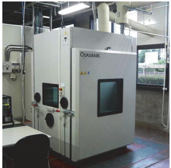
Figure 3 External View of HALT chamber
