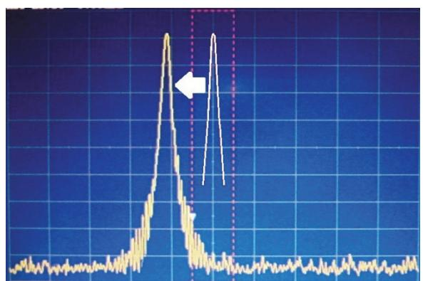
Figure 8 Unlocked Signal Drift (Span = 5 kHz)
