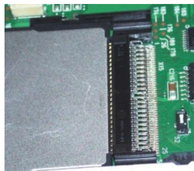
Figure 12 CF Card Slipping from Connector
