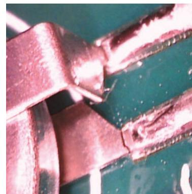
Figure 11 Fractured Backup Battery Lead
