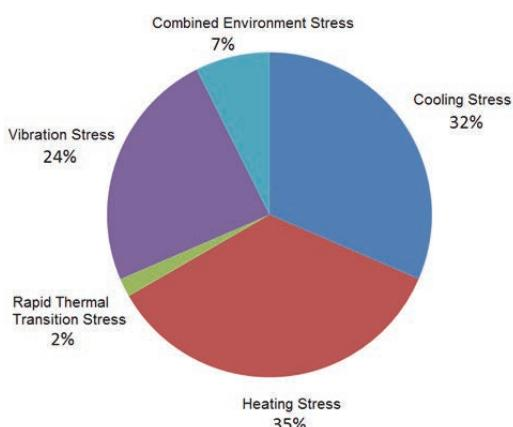
Figure 14 Faults Found by HALT
