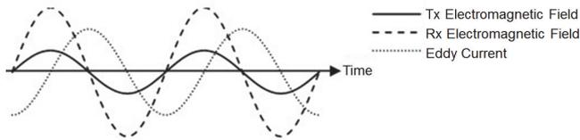
Figure 3 Relationship between Magnetic Field and Eddy Current
