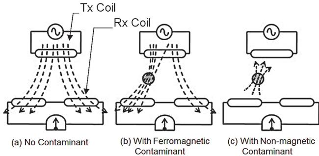
Figure 2 Principle of Metal Detector
