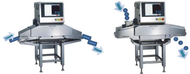
Figure 19 External View of X-ray Leak Prevention Mechanisms
