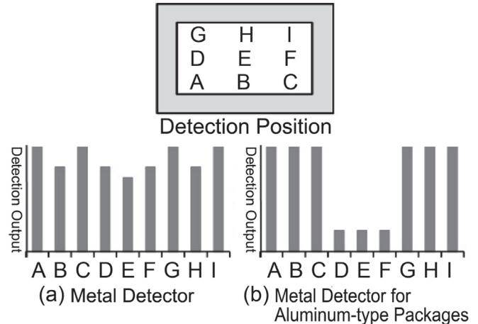
Figure 6 Relationship between Detection Sensitivity and Position
