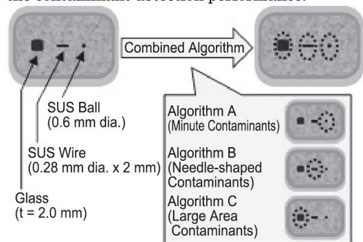
Figure 13 Concept of Combined Algorithm
