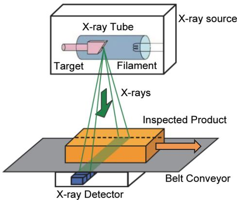
Figure 11 Principle of X-ray Inspection Systems
