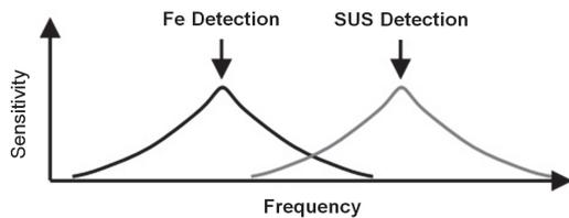
Figure 4 Relationship between Magnetic Field Frequency and Signal Levels
