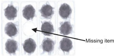
Figure 17 X-ray Image for Missing Product Detection
