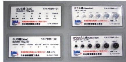
Figure 20 External View of Test Pieces for X-ray Inspection System
