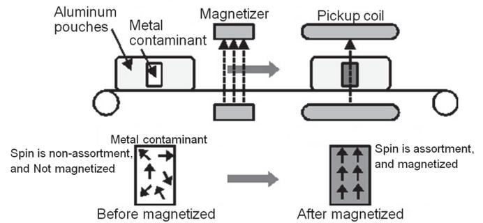
Figure 5 Detection Principle of M Series Metal Detector
