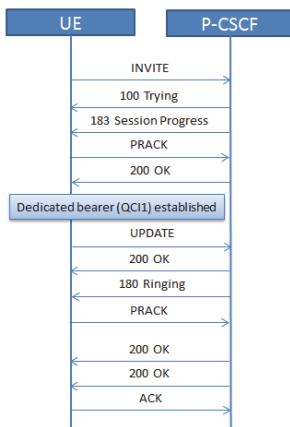
Figure 3 Mobile Origination Procedure
