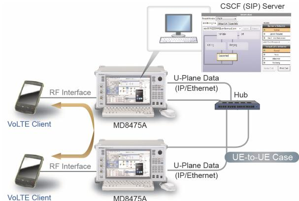
Figure 10 End-to-End Communicating Test
