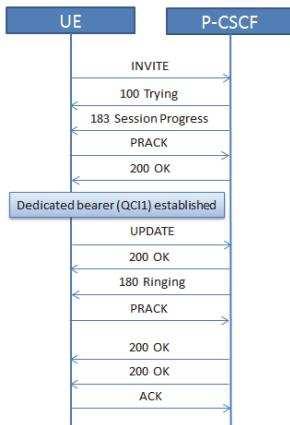
Figure 3 Mobile Origination Procedure
