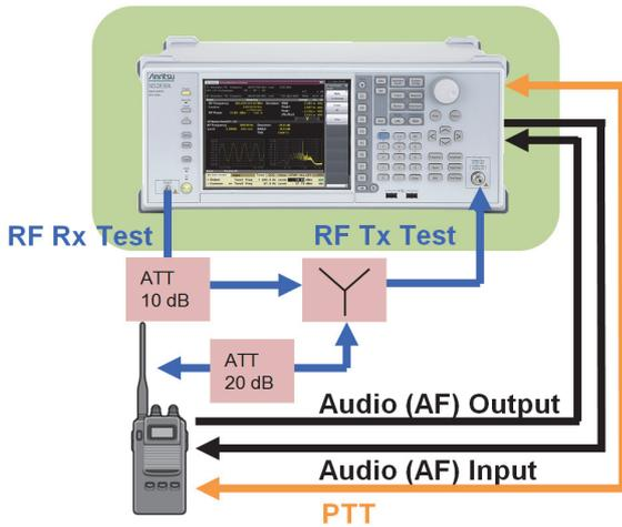
Figure 2 Measurement Concept Diagram with MS2830A-018 Installed
