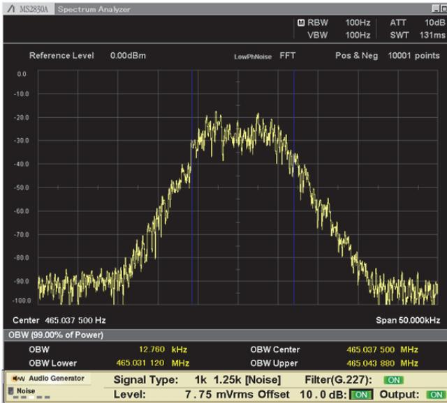
Figure 10 Occupied Frequency Bandwidth Measurement Screen
