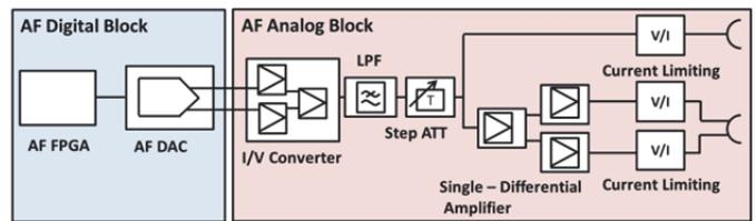
Figure 4 Audio Generator Block Diagram
