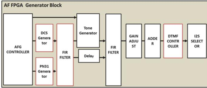
Figure 5 FPGA Signal Generator Block Diagram
