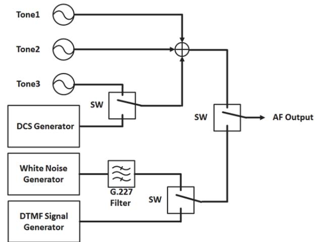
Figure 9 Audio Generator Concept Block Diagram
