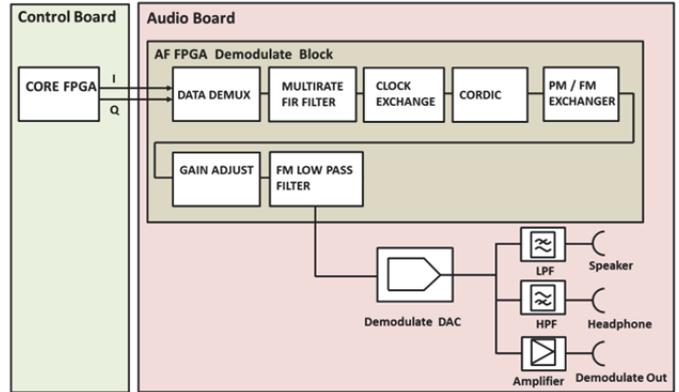
Figure 7 FM Demodulation Section
