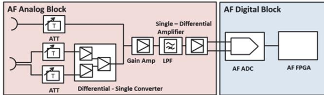
Figure 6 Audio Analyzer Block Diagram
