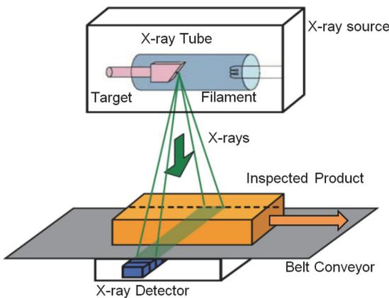
Figure 2 Principle of X-ray Inspection System
